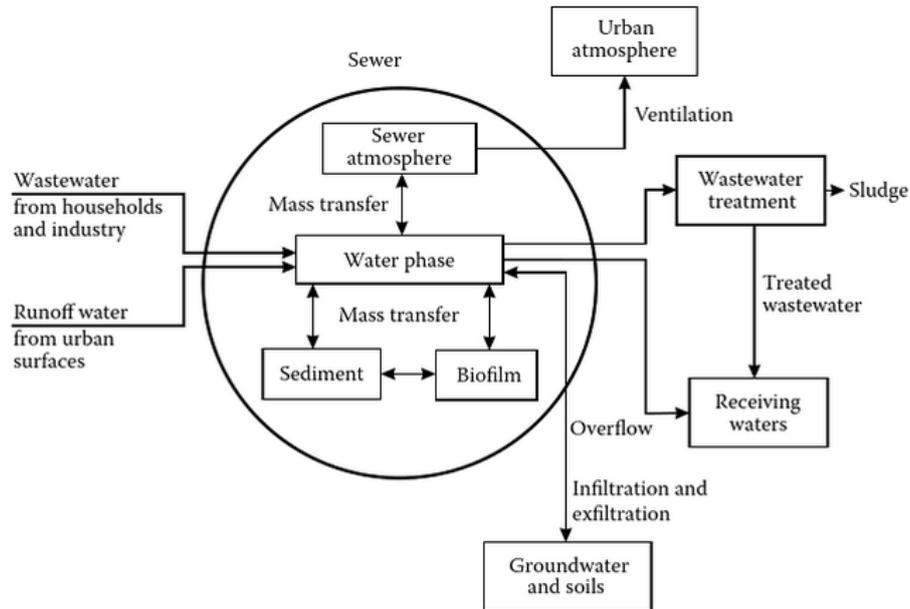
Figure 2: Sewer subsystems (phases) for the potential occurrence of sewer processes and wastewater flows between the sewer and the surrounding (urban) environment (Hvitved-Jacobsen et al., 2013).
