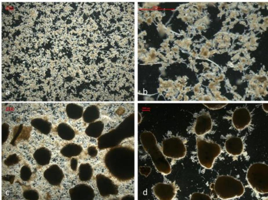
Figure 1: Sludge from the full-scale Nereda<sup>®</sup> reactor in Garmerwolde, the Netherlands. a) and b) biomass on top of the granular sludge bed; c) mixed liquors; d) granules sieved and washed with tap water. (M. Pronk, de Kreuk, et al., 2015)
