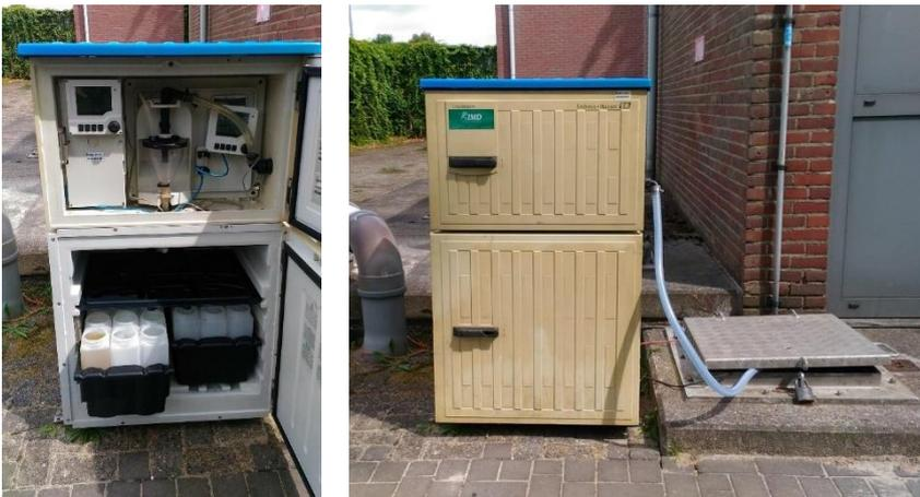
Figure 7: Automated vacuum sampler installed at the upstream location of the pressure sewer.
