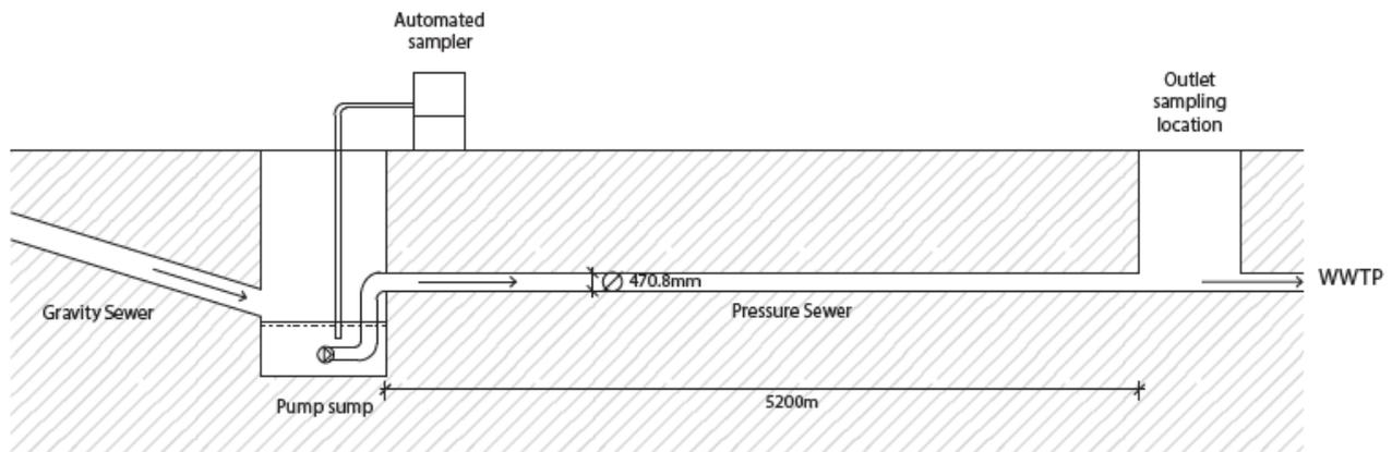
Figure 5: Schematic representation of the sampled pressure sewer (not to scale). The pressure sewer was made of a PVC pipe, with length and internal diameter reported in the figure. Sampling always occurred at the same times (10:00 and 14:00 during weekdays), with an average flow during sampling of 80 m<sup>3</sup>/h reaching the WWTP.
