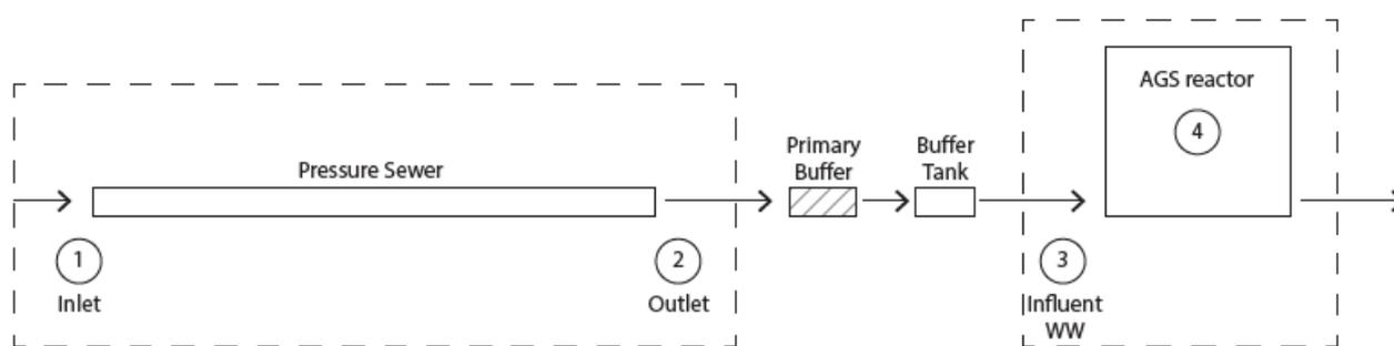
Figure 4: Schematic overview of the sampling locations in reference to the urban wastewater system. Note that the selected pressure sewer and AGS reactor were not part of the same system.
