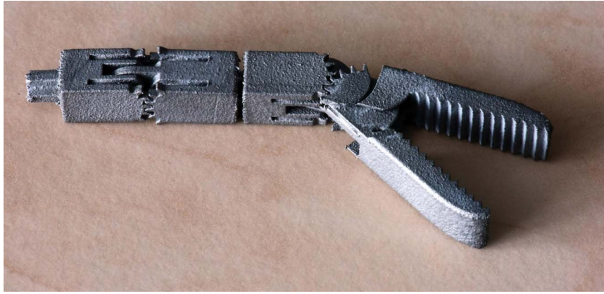
Fig. 1. Rolling toothed joint fabricated by AM.
