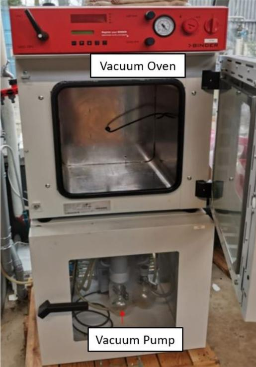
Figure 3.6: Vacuum Oven used for vacuum treatment of pressboard and paper
