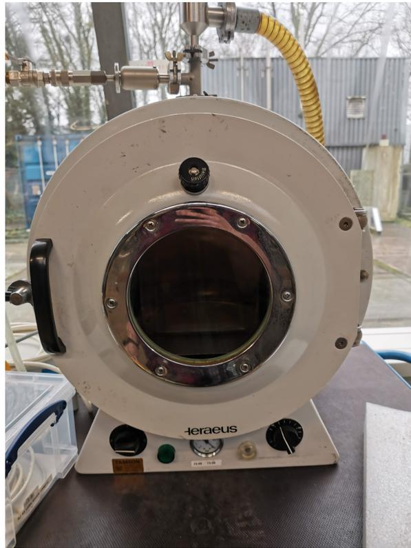
Figure 3.7: Vacuum oven used for degassing and vacuum treatment of oil
