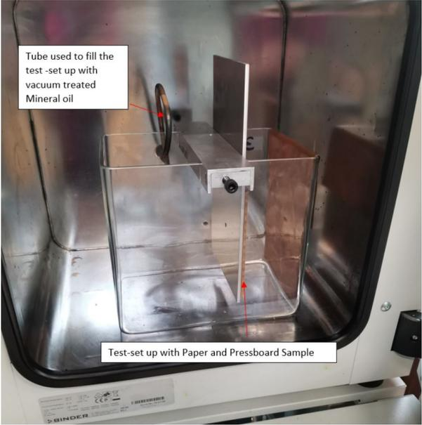
Figure 3.5: Test set with sample paper-pressboard is kept in vacuum oven
