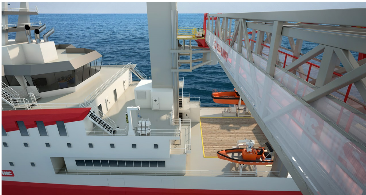
Figure 5.1: Example of a motion compensated gangway (Royal IHC, 2020a).
