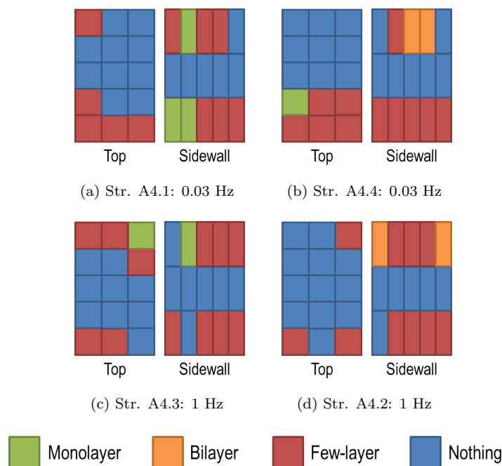
Figure 10.11: Schematics of the number of graphene layers of the top and one sidewall for structures from die A4. During deposition, the polarity was changing with a frequency of 0.03\ \text{Hz} or 1\ \text{Hz} .
