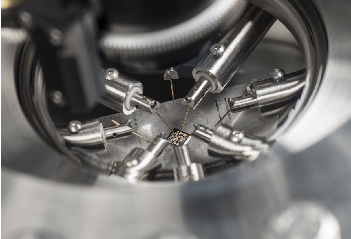
Figure D.2: Detailed picture of the probe station with a chip inside
