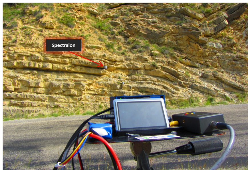
Fig 5. Positioning of the multispectral camera with respect to a rock formation including the Spectralon placed on the wall of the rock.
