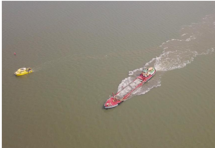
Figure 2: Turbidity plume introduced by dredging activities in the Waddenzee.
