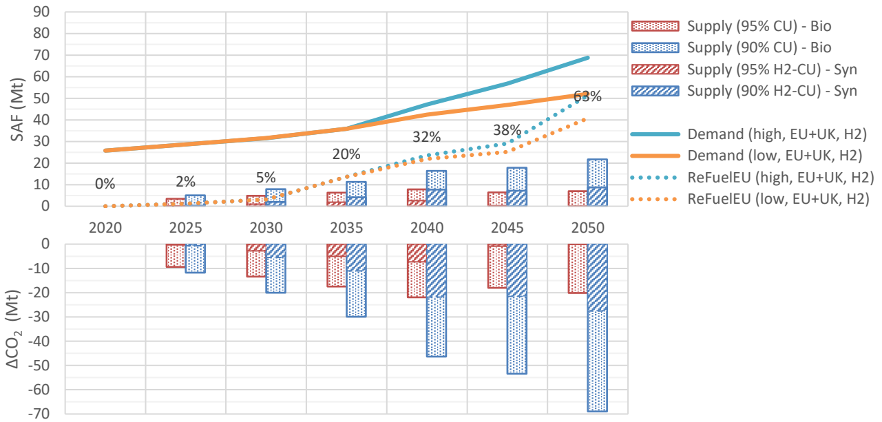
Figure 4 - Drop-in SAF demand based on technological and regulatory fleet-based blending limits (solid lines) or ReFuelEU mandate (dotted lines) and drop-in SAF supply (split in bio-based SAF supply and synthetic SAF supply) for flights departing from EU and UK (top). Net CO 2 emissions reduction based on the drop-in SAF supply (bottom). Results are shown for (low, high) traffic scenarios, for different cases of biomass and hydrogen competing use (CU), and with feedstock supply from the EU and UK and limited imports.
