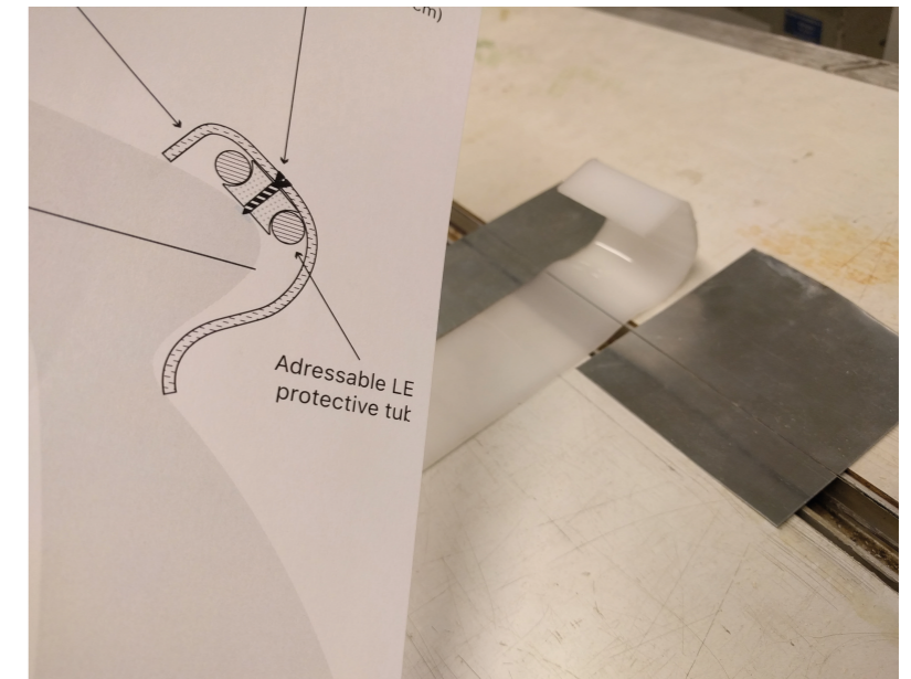
Figure J.2: Bending (only for prototyping) of the cover (small part ~50mm). Real length is the same as the length of the MX3D bridge handrail.
