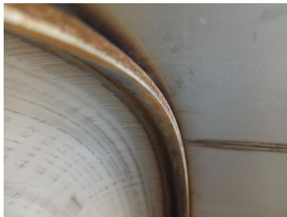
**Figure 3.12:** Photo of the welded joint between the half sphere and the cylinder that together make half a tank (flexible support test setup).
