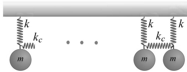
Figure 3. Locally resonant metastructures with internally coupled resonators
