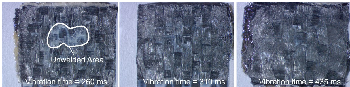
Figure 6: Representative fracture surfaces of joints obtained at (a) 260 ms (left), (b) 310 ms (middle) and (c) 435 ms (right) vibration times in Figure 4 [18].
