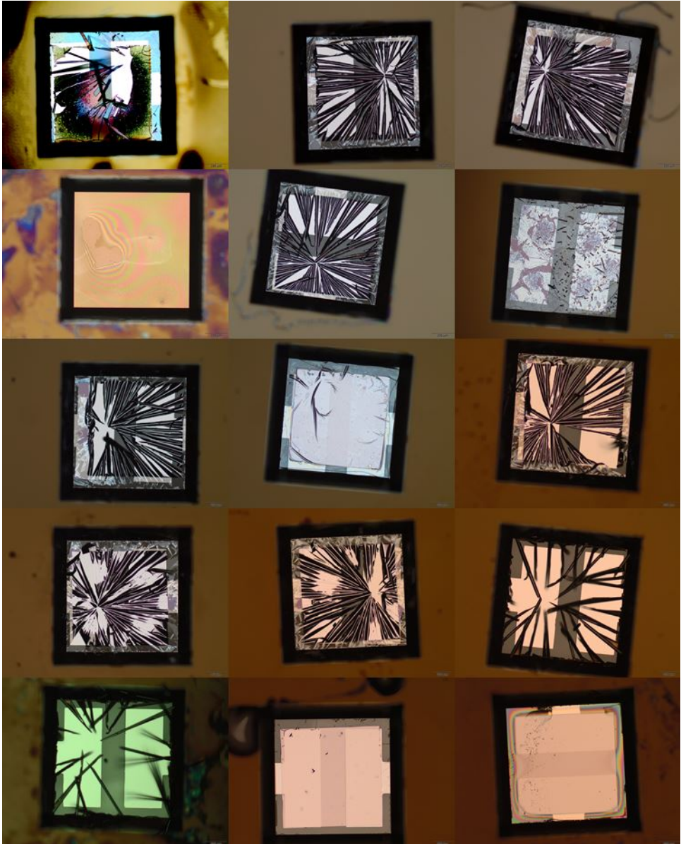
Figure 3.10: A visual demonstration of the fragility of the flip-chip method. This is a sample of the 40 Norcada chips that were flipped within this PhD.
