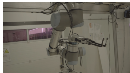
Picture 16: Robot capable of transplanting the plants from a Vertical Farm Tray at Logiqs
