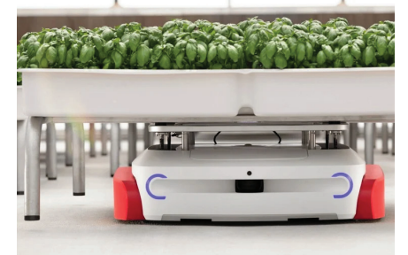
Picture 63: Bionic Hydroponic's cart robot carrying trays of plants (Bionic)
