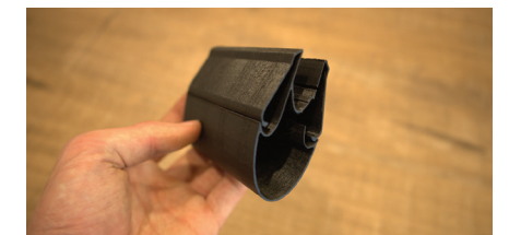
Picture 33: 3D print of gutter with included ventilation
