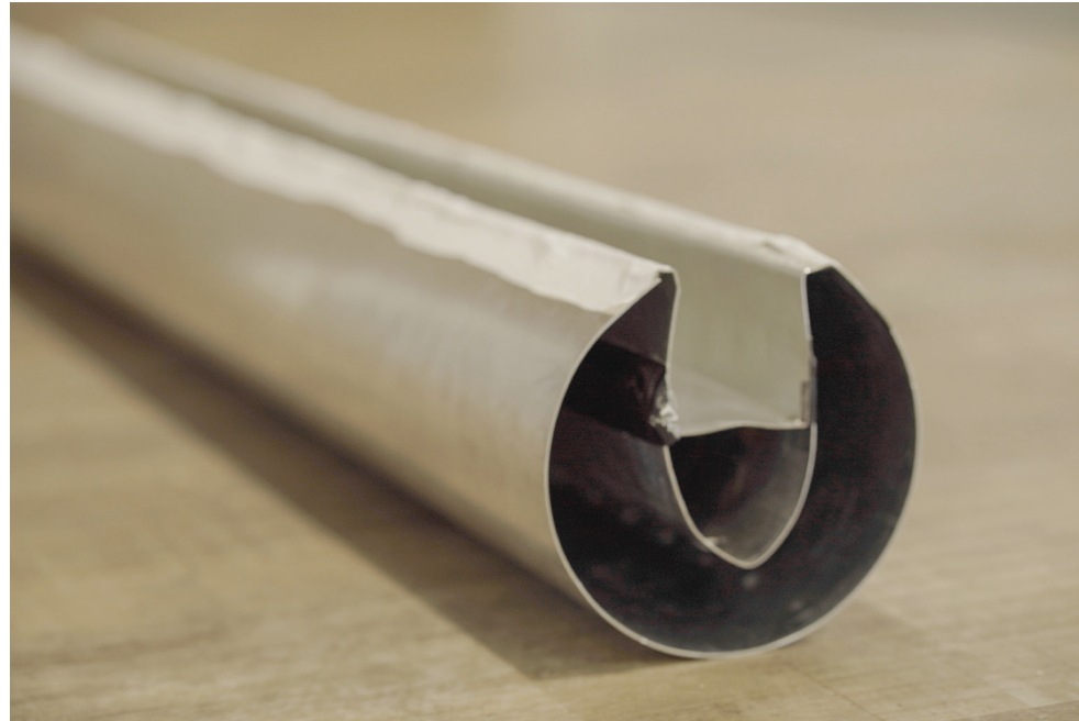
Picture 43, 44, 45: Hollow gutter prototype, Prototype with plants and ventilation, Perforations from the top view of the gutter
