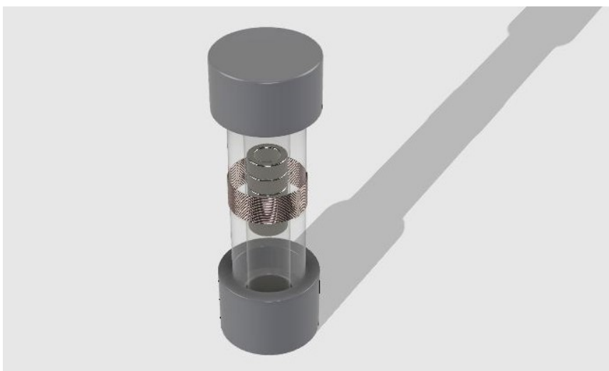
FIGURE E.12: 3D render of the designed motion energy harvester made in Autodesk Fusion 360
