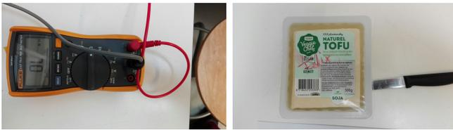
(a) FLUKE 117 Multimeter was used to measure the resistance of tofu (b) *JUMBO Veggie Chef Naturel Tofu* used in experiments
