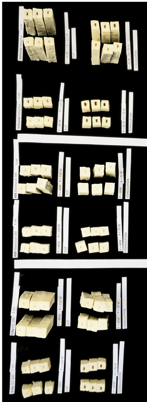
Fig. G.9: Photo of all test samples after conducted experiments. Using the Burn Scale in Table IV these samples were analyzed and included in all Thermal Camera Test tables such as Table VII and VIII
