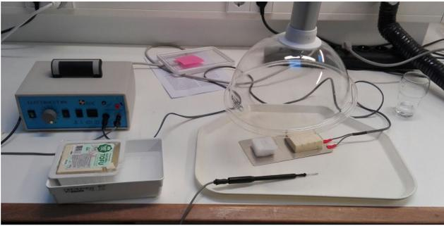
Fig. E.3: Experimental set-up to test if PVA or tofu is a better material to replace animal tissue in a electrosurgical thermal test.
