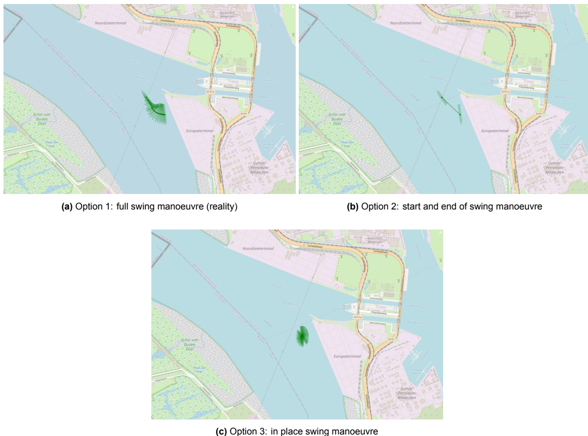
Figure 4.11: Different options for modelling a swing manoeuvre
