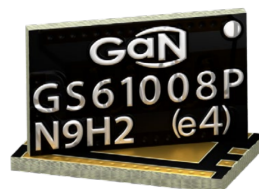
Figure 6.24: The figure of GS61008P 100V GaN enhancement-mode HEMT from GaN Systems.
