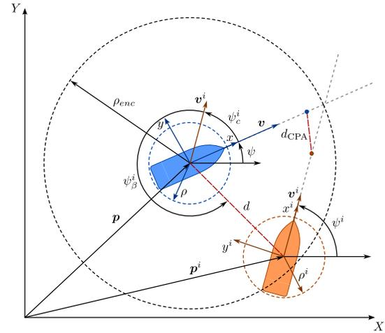
Fig. 3. Encounter situation analysis between the ASV and OV  $i$ . Their current states  $\mathbf{z}(t)$  and  $\mathbf{z}^i(t)$  are used to determine the distance at the Closest Point of Approach ( $d_{\text{CPA}}$ ) and thus if risk of collision exists assuming constant velocities.
