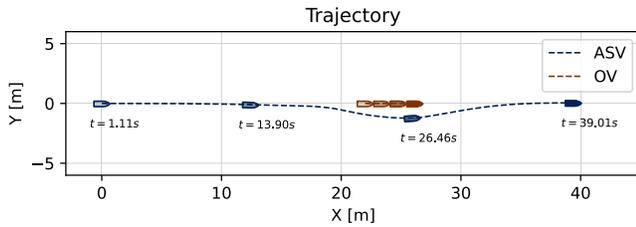
Fig. 9. Overtaking situation with the ASV in GW role, turning to starboard while it keeps out of the way of the OV (Rule 13).
