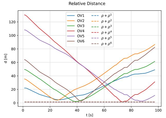
Fig. 19. The distance between the ASV and each OV in the scenario presented in Figure 13 as a function of time. The lower dashed line represents the sum of  $\rho + \rho^i$  for each OV showing that there is no collision.
