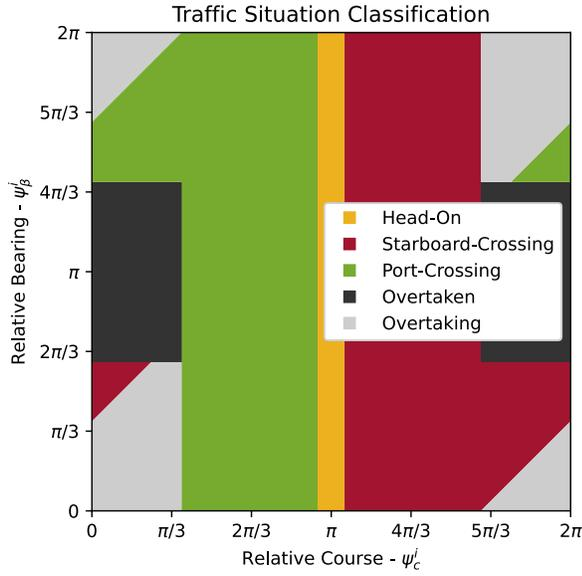
Fig. 4. Traffic situation classification as a function of the relative course  $\psi_c^i$ , and the relative bearing  $\psi_\beta^i$  described in [6]. Note that the same figure from the perspective of the OV would be role-symmetric since pairwise-role symmetry is necessary.
