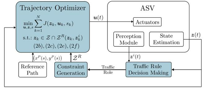
Fig. 1. Schematic method overview (light blue blocks). Given the measured states  $\mathbf{z}(t)$  and  $\mathbf{z}^i(t)$ , we first infer the traffic role of the vessels based on which a suitable set of constraints is generated. The latter is then inserted in the optimization problem and the first step of the optimal input sequence,  $\mathbf{u}_1^*$ , is applied to the ASV at each control cycle as  $\mathbf{u}(t)$ .
