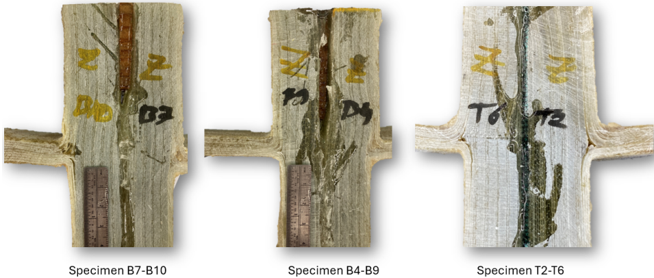
Figure 4.9: Fatigue failure mode
