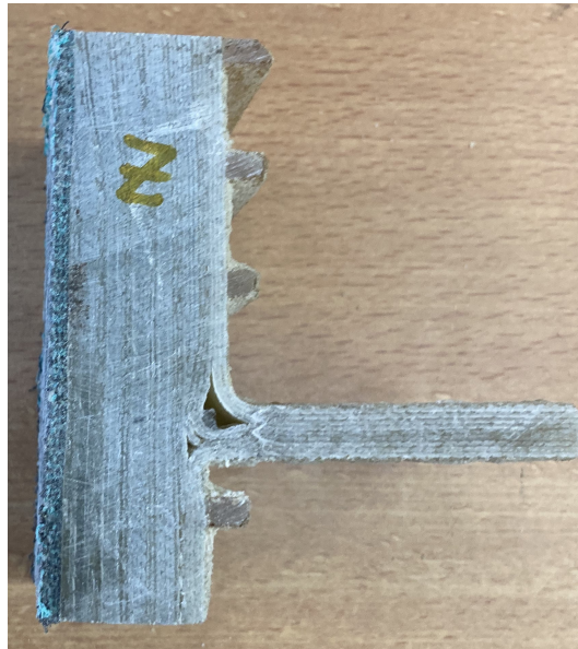
Figure 3.9: Specimen T12, with imperfection rating 2 and a web thickness of 10.53 mm
