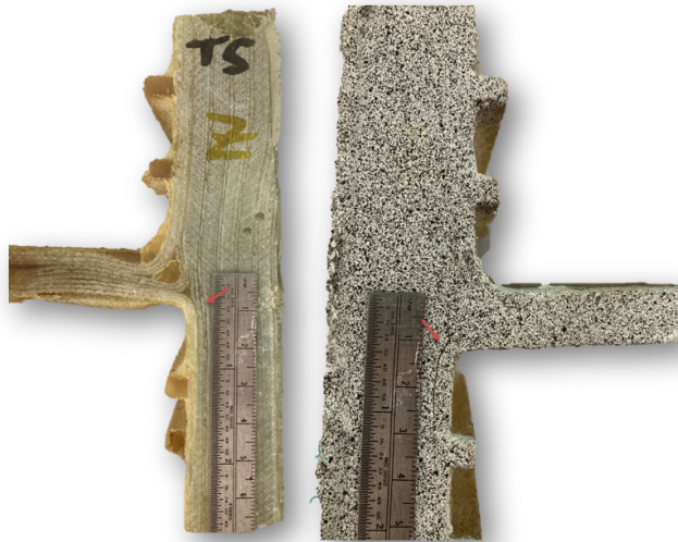
Specimen T5 with cracks
