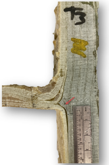
Specimen T3 with crack
