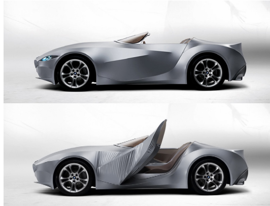
Figure 67. The GINA Light Visionary Model is a fabric-skinned shape-shifting sports car concept built by BMW
