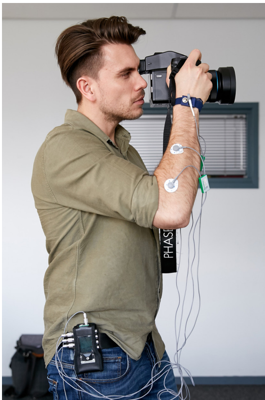
Figure 60. Participant holds the camera in an active state during an EMG measurement.
