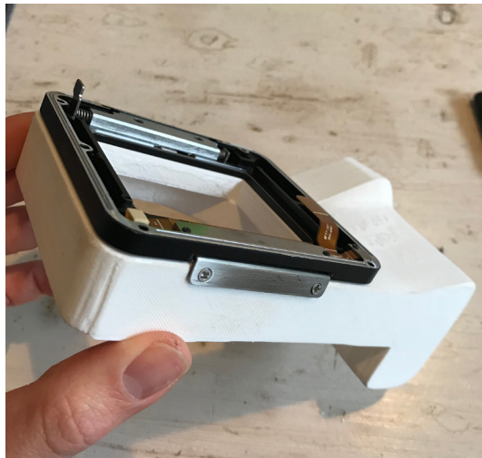
Figure 56. A mounting plate from a Phase One digital back can thereby be fitted to the the printed model.
