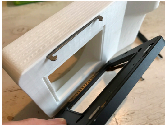
Figure 55. Metal brackets, Phase One spare parts, were mounted in the 3D printed models.
