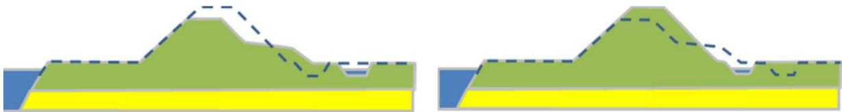
**Figure 3.5:** An overview of two different designs with an equal probability of failure. The design with height as dominant failure mechanism results in a lower and wider dike, while a design with stability as dominant failure mechanisms results in a higher and smaller dike (Knoeff, 2016).
