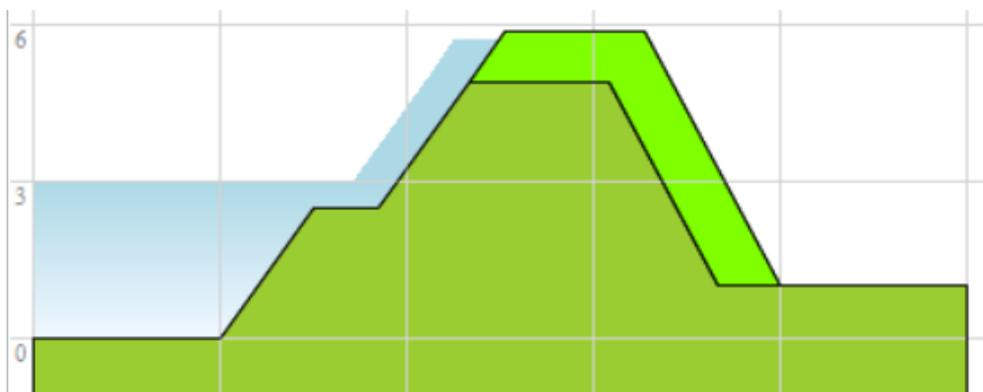
**Figure E.3:** Cross section of an example of reinforcing profile 3. In this cross-section, the increase in crest level is 0,96 m. On the left side is the river located.
