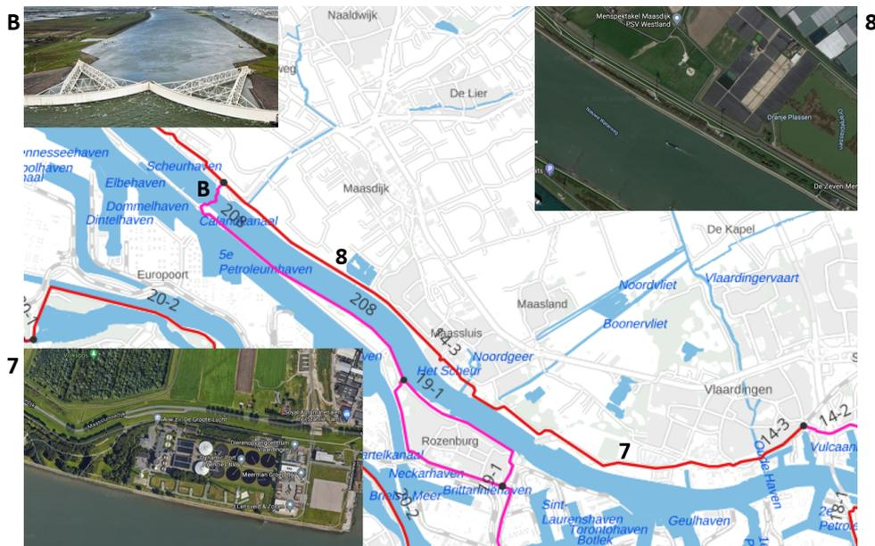
**Figure 3.10:** An overview of the locations of the two assessed cross sections (7 and 8) in trajectory 14-3 and the location of the Maeslantbarrier (B) in dike trajectory 14-3. Location 8 does not have foreland and location 7 does.
