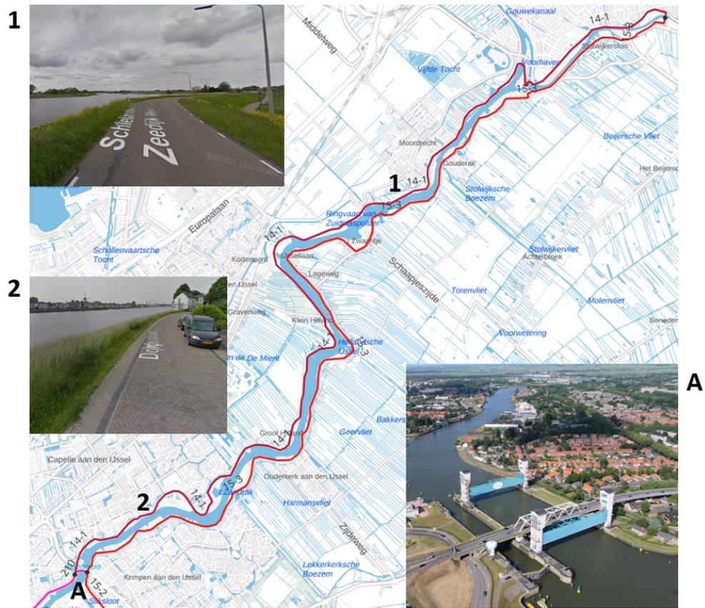
**Figure 3.8:** An overview of the locations of the two assessed cross sections (1 and 2) and the location of the Hollandse IJssel barrier (A) in dike trajectory 14-1. Both locations do not have foreland.
