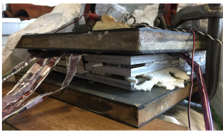
Figure 7.11: Tile mold bursting open during curing of sample R3-TM1-1
