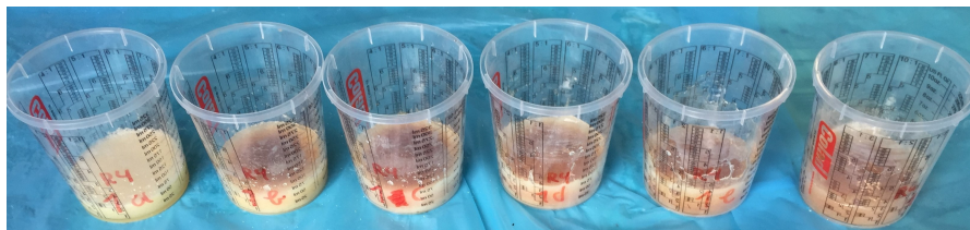
(a) All cured mixtures on a row: used epoxy mix ratios from left to right; 1a) 100:10, 1b) 100:20, 1c) 100:30, 1d) 100:40, 1e) 100:50 and 1f) 100:60
