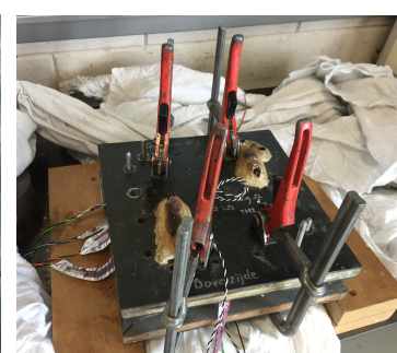
Figure E.3: Closed tile mold using 4 glue clasps.
