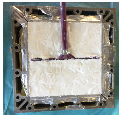
Figure 7.9: Sample casing filled with EX-CORE and sensor grid positioned at mid plane
