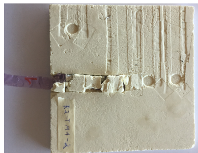
Figure 6.12: Cured sample R2-TM1-2. Cut outs made to free NTC sensor
