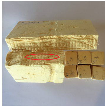
Figure 8.2: Sample R4-TM1-2; crack indicated
