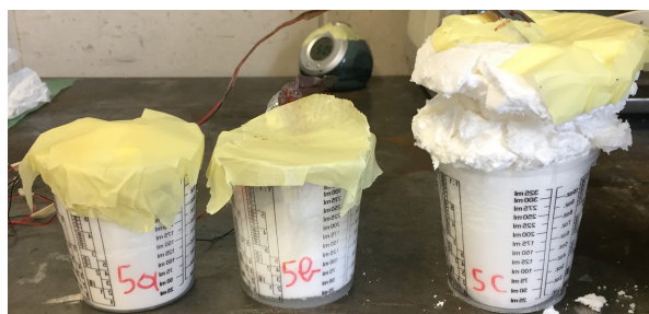
Figure 7.4: 031DU/water mixtures when cooled back to room temp. Composition: 5a) 50ml DU, 5b) 50g water & 2g 031DU and 5c) 50g water & 50g 031DU
