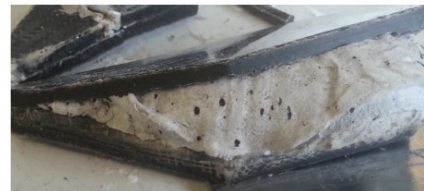
Figure 3.4: Re-expansion of Expancel ® DU/DE sample with CF/epoxy facings after reheating at 105°C [58]
