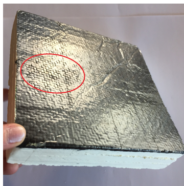
Figure 10.6: Sample R8-TM1-1 (bottom surface), dry area with rel. large amount of surface porosity indicated
