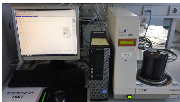
(a) Seiko Instruments Exstar 6000 DSC and computer used for data collection
