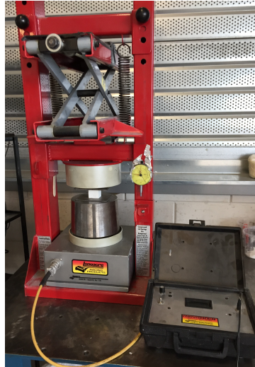
Figure 8.9: Donkervoort's pressure jack with load cell, dial gauge micrometer and readout display.
