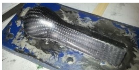
Figure 3.6: Gear knob produced in one shot with DU/DE/epoxy core mixture and CF/epoxy facesheets [58]
