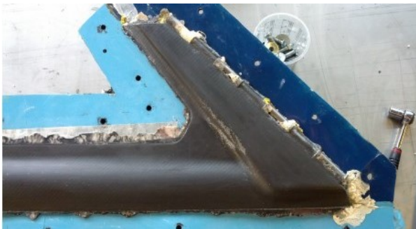
Figure 3.7: Door beam with low amount of surface porosity produced with PET foil between core and CFRP prepreg facings [60]
