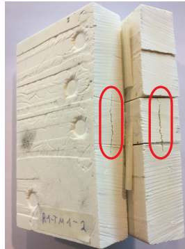
Figure 6.7: Cross-section of sample R1-TM1-2. Crack indicated.
