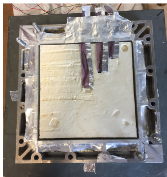
Figure 6.10: Shrunken sample R1-TM1-6 after heating in 130°C mold
