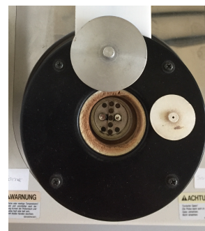
(b) DSC test chamber and furnace of the Seiko Instruments Exstar 6000 DSC
