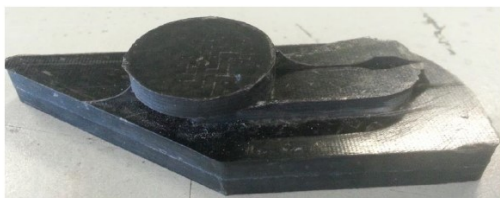
Figure 3.5: Complex shaped demonstrator sandwich structure produced in one shot with DU/DE/epoxy core mixture and CF/epoxy facesheets [58]
