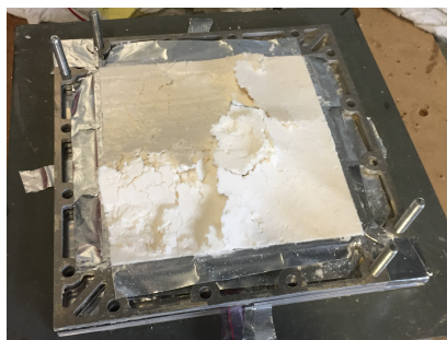
Figure 6.11: Brittle sample R2-TM1-1, bursting out of mold when opened.
