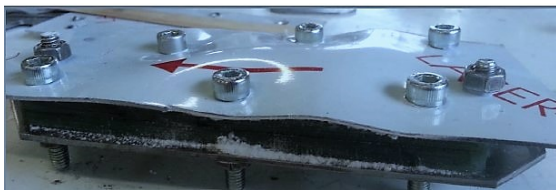
Figure 3.3: Deformation of 1.3mm aluminum mold lid after curing of Expancel ® 7:1 DU/DE mix [58]
