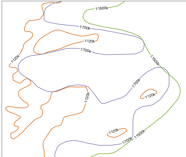
Figure 2.6: The same isobath generalised at different scales. Deeper parts of the seabed are on the right side of the figure. From large scale (orange), medium scale (purple) to small scale (green). Data from NOAA
