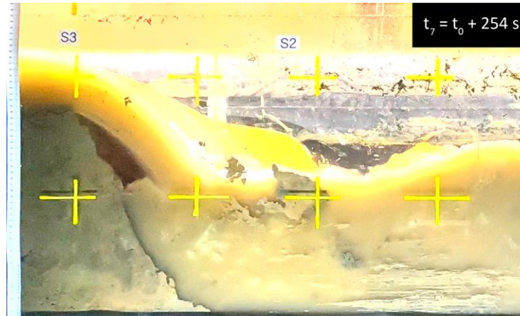
Figure 4.11: RC3 GoPro 2 snapshot at t_7 = t_0 + 254 seconds ( t_6 + 1 second). The eroded block has been pushed one meter downstream. The downstream water level increases and an aerated nappe arises at the newly formed headcut.
