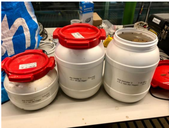
River clay sample containers for the sediment analysis. The containers were stored in a cooled climate room.
