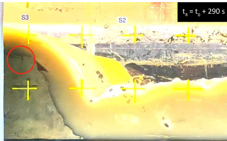
Figure 4.12: RC3 GoPro 2 snapshot at t_8 = t_0 + 290 seconds ( t_7 + 36 seconds). During this time headcut erosion occurred. The eroded block is washed away and therefore the downstream water level decreases. A new crack formation is indicated with the red circle. The block erosion process repeats.
