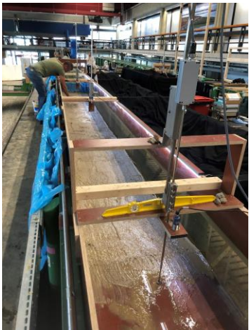
Final condition of the river clay package before the start of the experiments.
