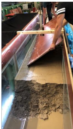
Figure 2.3: Image of placing the concrete plywood panels on top of the river clay package.
