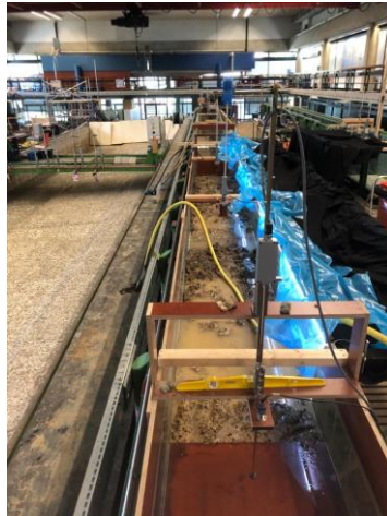
Position and installation of the EMS, MIC 1-3, and preparation of the river clay package.
