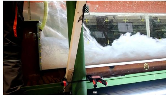
Aerating of the depressed nappe cavity through the aeration tube during the experimental setup test run.
