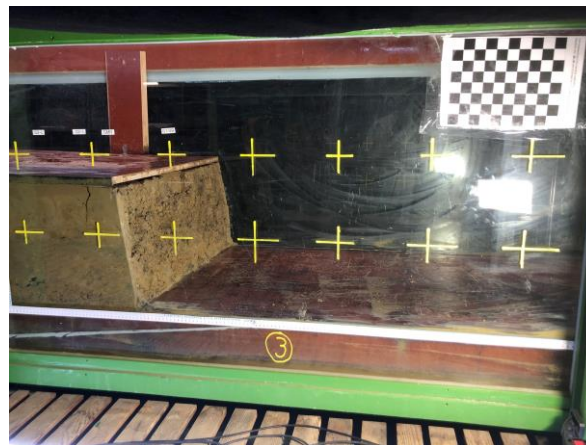
Figure 2.4: Side view image of the Tompouce experimental setup taken at the headcut location. The false bottom and yellow plus-grid can be observed as well.
