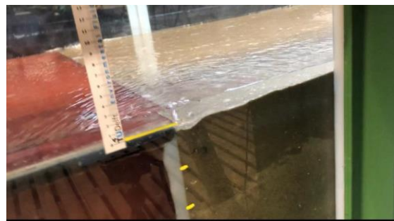
Close-up of the scour hole development at the broad-crested weir material transition during a North Sea sand experiment.
