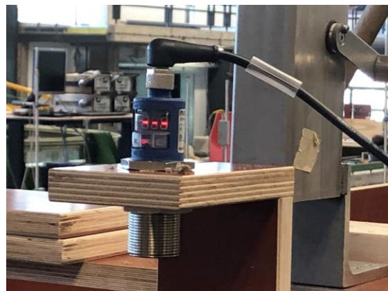
Installation and mounting of the ultrasonic echo sensor (type MIC+35).
