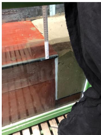
Scour hole development at the broad-crested weir during a North Sea sand experiment.
