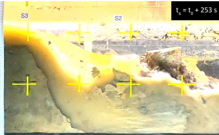
Figure 4.10: RC3 GoPro 2 snapshot at t_6 = t_0 + 253 seconds ( t_5 + 1 second). The block has become completely detached and is pushed further downstream by impulses of water flow.
