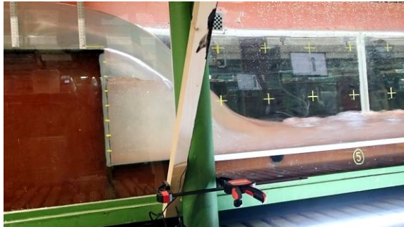
Depressed (non-aerated) nappe during experimental setup test run.
