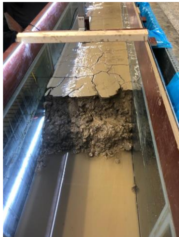
River clay headcut after removing of the Tompouce setup. The surface cracks are clearly visible.
