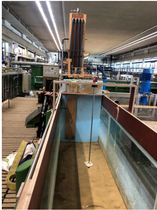
Installation of the MPS 1 upstream of the broad-crested weir.
