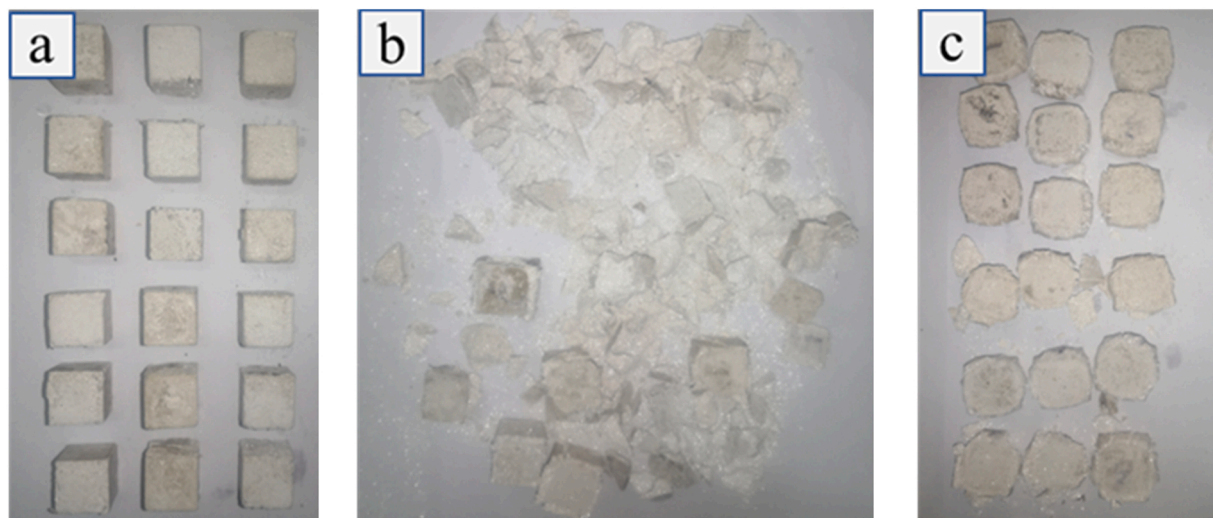
Fig. 8. Compressive sample diagram (a. before test; b. after 23 °C; c. after 50 °C).
