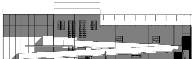
Fig. 1 Section with the long ramps
