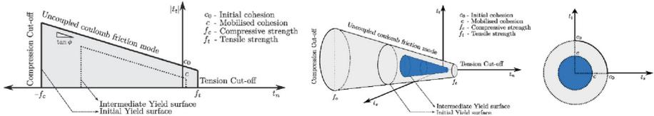
**Fig. 1.** Failure surface for the 2D line interfaces (left) and 3D planar interfaces (right)
