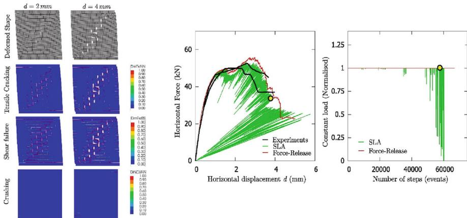
**Fig. 4.** The deformed profile, and damage plots indicating tensile, shear and crushing failures for the pushover study, with discrete cracking-shearing-crushing interfaces, using the SLA method at 2 mm and 4 mm prescribed lateral displacements. Force–displacement curves of the experiments compared against those of the SLA and the Force-Release simulations, and (b) the evolution of constant load of pre-compression during the simulations.
