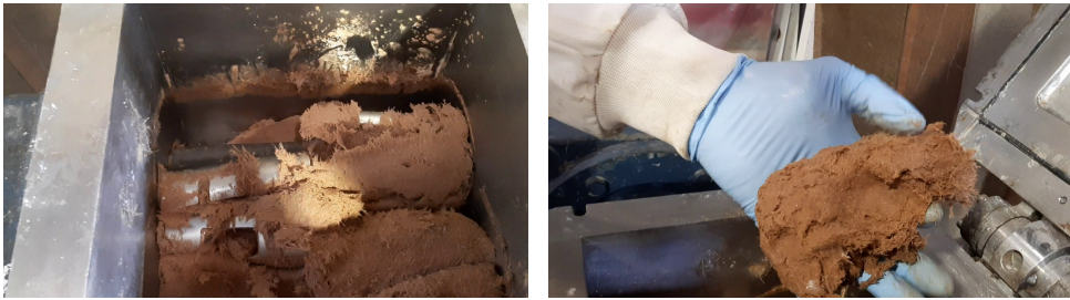
Figure 3.4: Bio-based composite bulk moulding compound (BMC) from Recell fibre and peach stone/calcite fillers.
