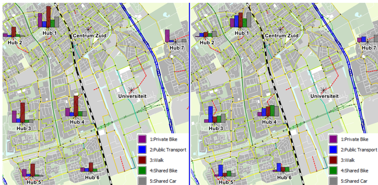
Figure 32: Representation of arrivals at mobility hubs by different modes (left), departures from mobility hubs by different modes (right) on OmniTRANS
