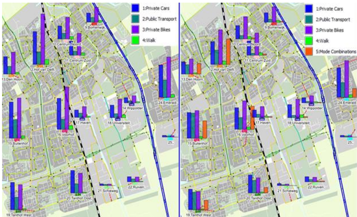
Figure 28: Representation of total trips departing from internal zones by different modes: without hubs (left), with hubs (right) on OmniTRANS.
