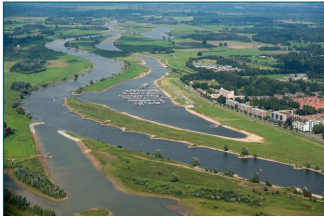
Figure 5.6 – Flood relief channels next to the river IJssel at the Zandweerd Pond (van Gerner, 2015)
