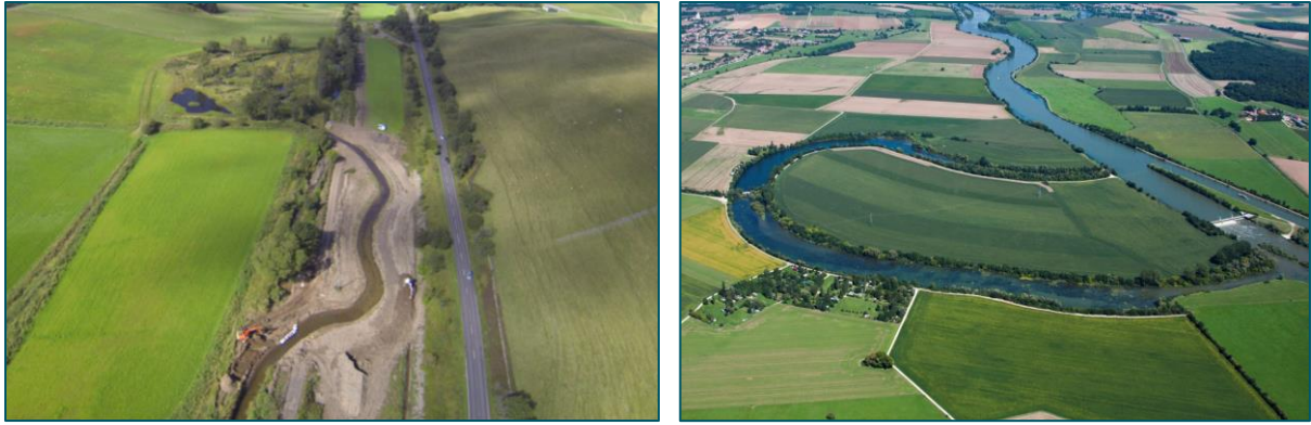
Figure 4.6 – (a) Re-meandering of a straightened river at the Eddleston Water, Scotland (Spray, 2022); (b) Reconnection of oxbow lake to main channel at the Saône, France (NWRM, 2013).
