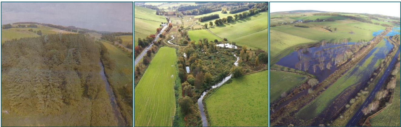
Figure 5.2 - – Pictures of “Lake Wood” at the Eddleston Water Project – (a) straightened river; (b) re-meandered river under normal conditions; (c) re-meandered river, storing water during a flood.
