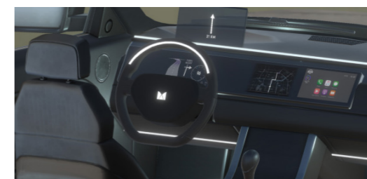
Figure 13 Depleting bar on the steering wheel (Shan, 2021)
