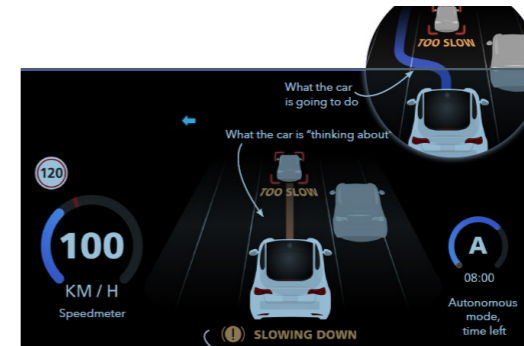
Figure 11 HMI communication and further explanation about the choice of the system (Wang, 2020)
