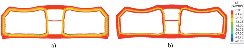
Figure 8. Principal compressive stresses for scenario B: a) plane strain and no spalling at 365 minutes; b) plane strain with explicit spalling at 72 minutes.
