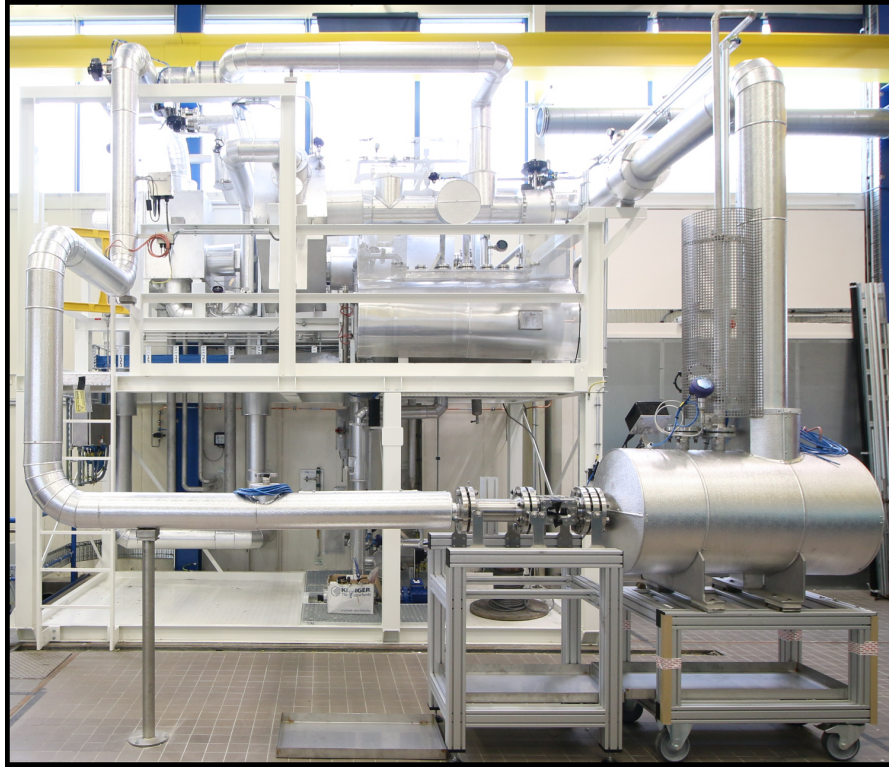
Figure 2.12: The ORCHID, in the bottom-right of the picture can be seen the nozzle window. Taken from Head [34].
