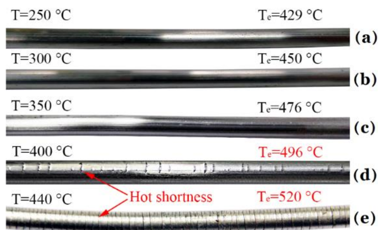
431 432 Fig. 8. Magnesium alloy rods extruded at a reduction ratio of 29.8, stem speed of 3.93 mm/s and 433 different billet temperatures. T_e is the maximum extrudate temperature. (a) T=523 K (250 °C) and 434 T_e=702 K (429 °C); (b) T=573 K (300 °C) and T_e=723 K (450 °C); (c) T=623 K (350 °C) and 435 T_e=749 K (476 °C); (d) T=673 K (400 °C) and T_e=769 K (496 °C); (e) T=713 K (440 °C) and 436 T_e=793 K (520 °C).
