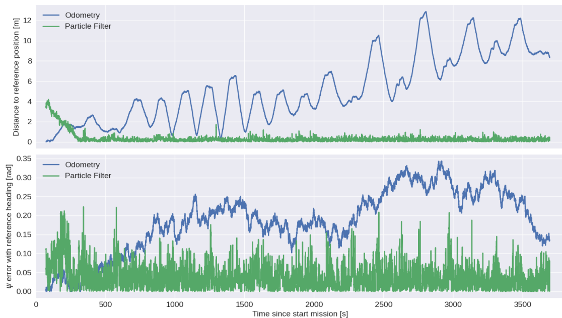
Figure 5-7: Distance of odometry and particle filter trajectories compared to the reference trajectory.
