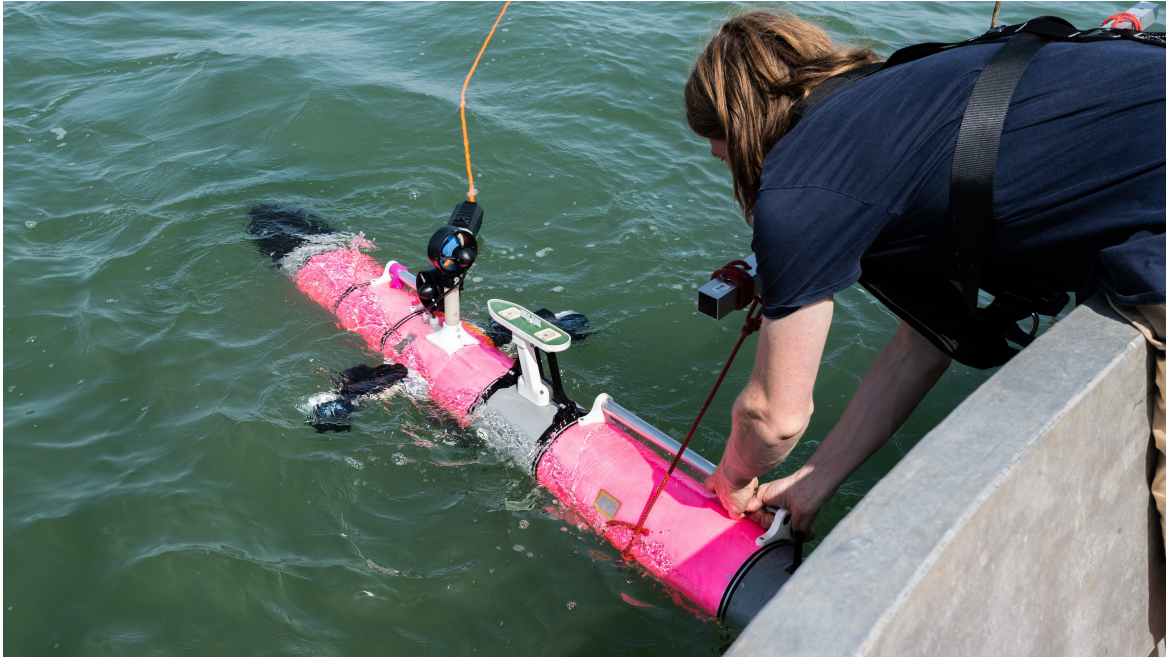
Figure 1-3: The Lobster Scout, the AUV used for experimental data collection for demonstration and validation of the proposed algorithms.
