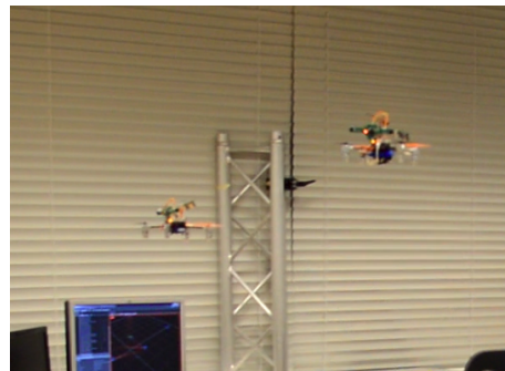
Fig. 1: Two pocket-drones (40 g each) flying autonomously in a real-world indoor environment using only on-board sensing and processing.
