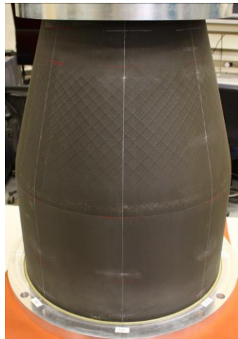
Figure 5. Test article potted in the end rings.
