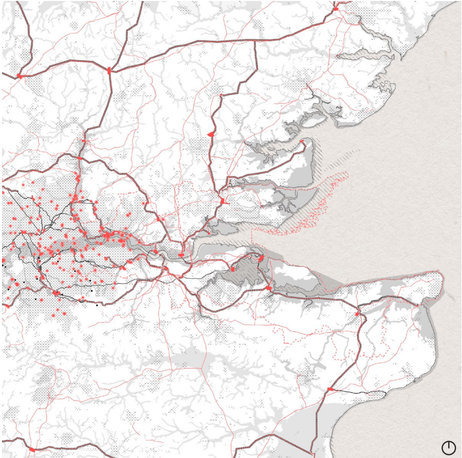
Figure 45 Utilities infrastructure at flood risk (includes electricity supply, gas, telecommunications, sewage and water supply), Source: Made by author, Data from Ordnance Survey, 2017
