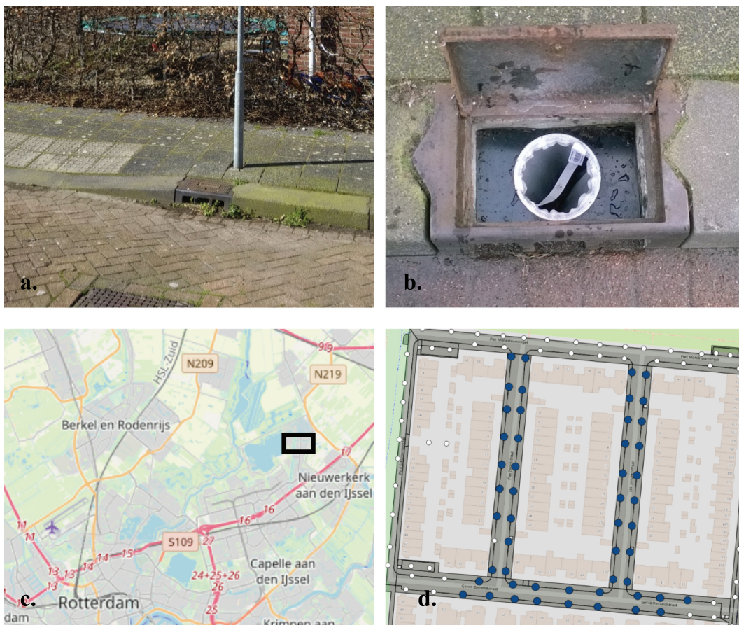
Figure 1. (a) Gully pot in the monitored streets. (b) Experimental set-up in the gully pot. (c) Map with rectangle indicating the monitoring area. (d) Street map of monitoring area in which the big blue dots indicate the selected gully pots and the small white ones gully pots not selected.
