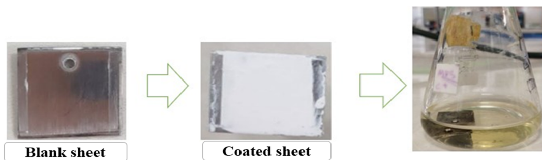
Figure 1. Preparation of metal sheets coated with paint–NP complexes for the antibacterial test.
