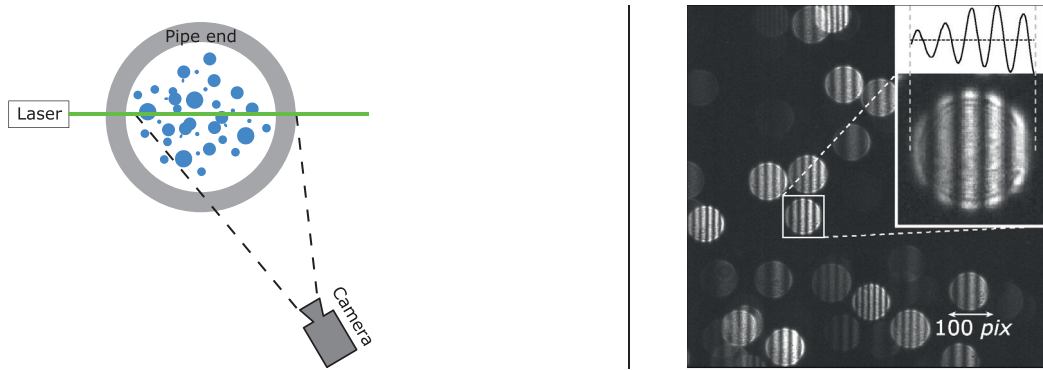
Fig. 10. Schematic representation of the IPI set-up (left) and a cut-out of a typical image obtained with this method (right). The insert shows the normalized interference pattern obtained from the enlarged droplet image after normalization and the application of a moving average filter.
