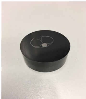
Figure 2.12: Sample mounted with conduction polyfast resin and polished.
