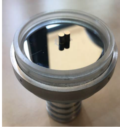
Figure 2.11: Schematic of the mounting of the sample on the Si wafer {510} for XRD measurement.
