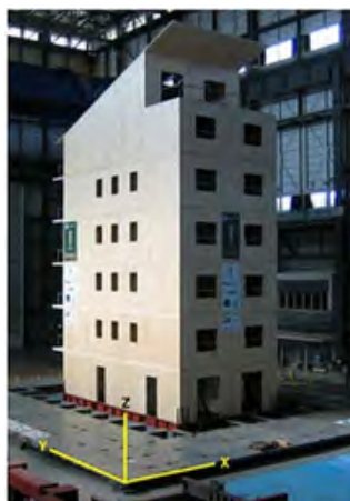
Figure 1.2.1: Full size Test of a 7 storey building made of CLT [12]
