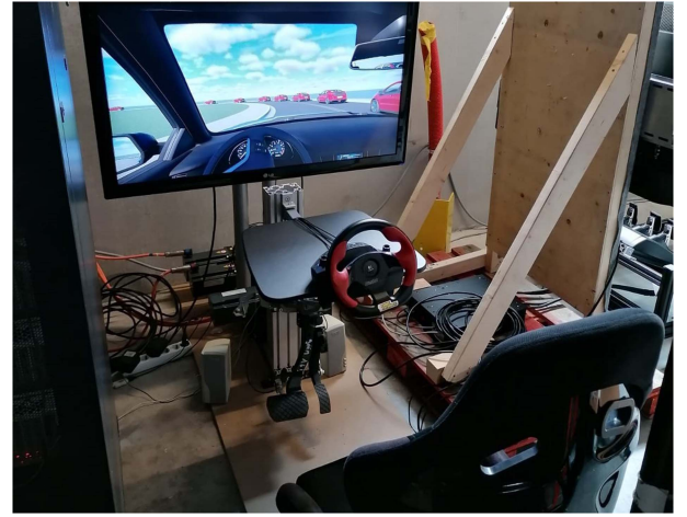
Fig. 3. Fixed-base driving simulator setup.
