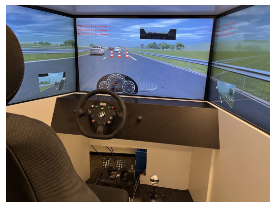
Fig. 1: A view from the driver's seat in the driving simulator.
