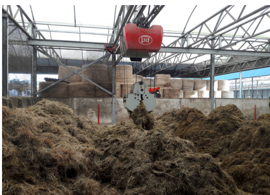
Figure 3.11: The feed robot at Hoeve Biesland automatically picks and mixes the fodder (Author)
