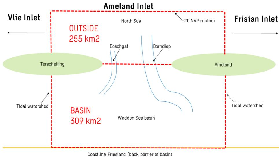
Figure 2.10: Sketch of outside and inside surface areas of the Ameland Inlet. The North Sea contour is closed by the -20NAP line. The tidal watersheds separate the Ameland Basin from the Vlie and Frisian Inlet. The nourishment requirements determined in Table 2.1 are based on the surfaces areas as depicted in this figure.
