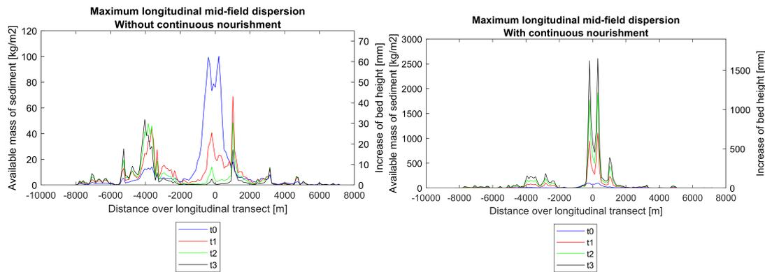
(a) The maximum dispersion over the longitudinal transect per fraction without the addition of a continuous nourishment over a half year. (b) The maximum dispersion over the longitudinal transect per fraction with the addition of a continuous nourishment over a half year.
