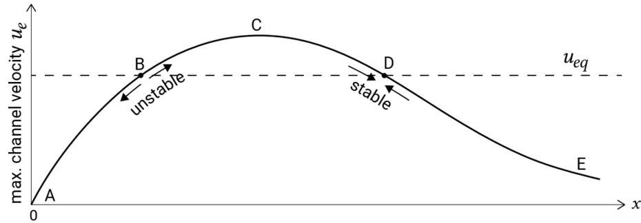
Figure B.2: Escoffier's maximum cross-sectional averaged entrance channel velocity  $u_e$  versus stable and unstable perturbations (Bosboom and Stive, 2021)
