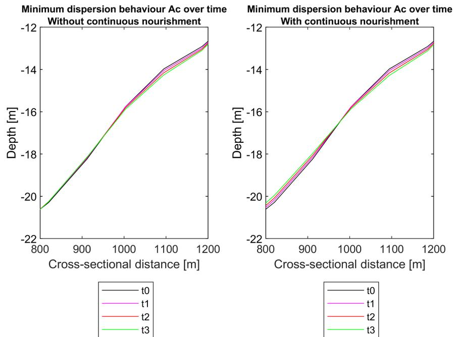
Figure K.3: Behaviour of cross-section over time with a continuous nourishment - Part 3
