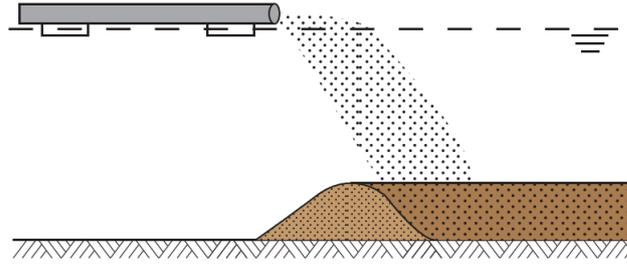
Figure L.1: Pipeline discharge on top of water column (van't Hoff and van der Kolff, 2012)
