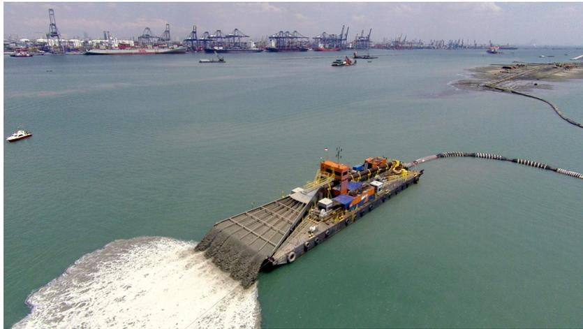
Figure L.3: Example spray pontoon
