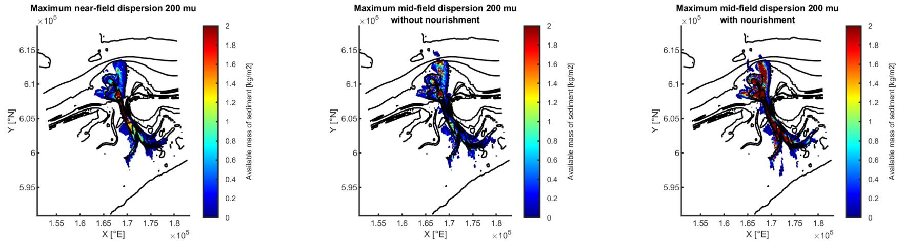
Figure 6.6: Combined figures of maximum dispersion. 3D spring neap tide cycle (left), 2D half year dispersion without continuous nourishment (center) and 2D half year dispersion with continuous nourishment (right) - 200 $\mu$ m
