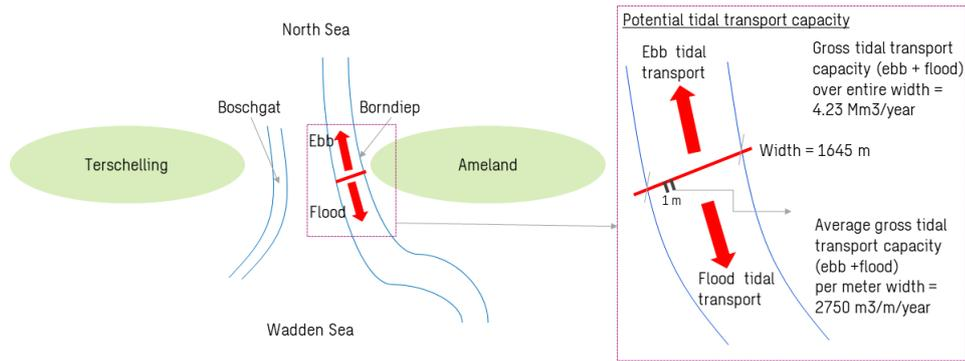
Figure 4.2: Overview of gross tidal sediment transport capacity of the Borndiep channel. This image also illustrates how the average gross tidal sediment transport capacity per meter is obtained.
