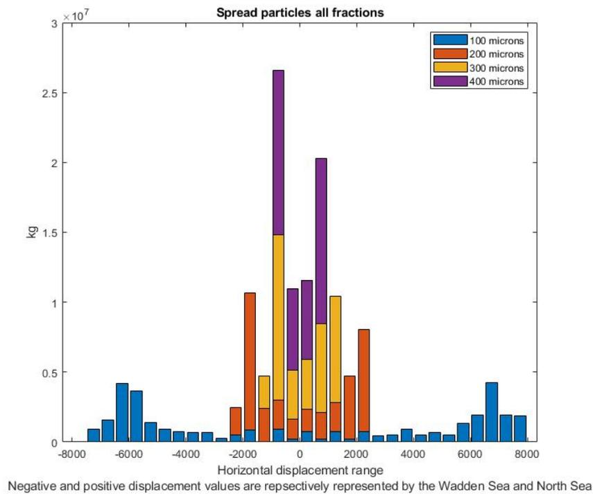
Figure I.11: Mass [kg] distribution of settling particles
