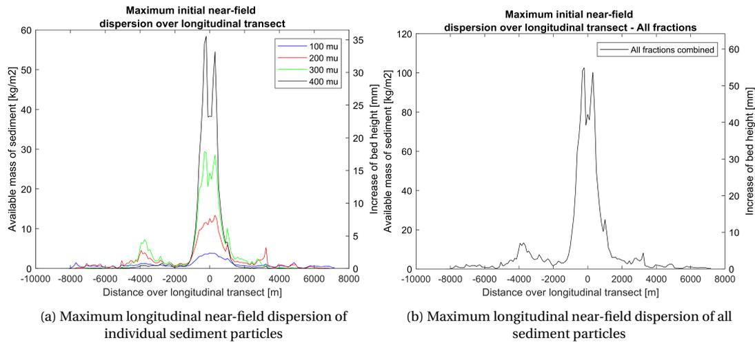
Figure 5.9: Longitudinal transect of maximum near-field dispersion. The longitudinal transect is taken through the tidal channel as depicted in Fig. 5.7a.
