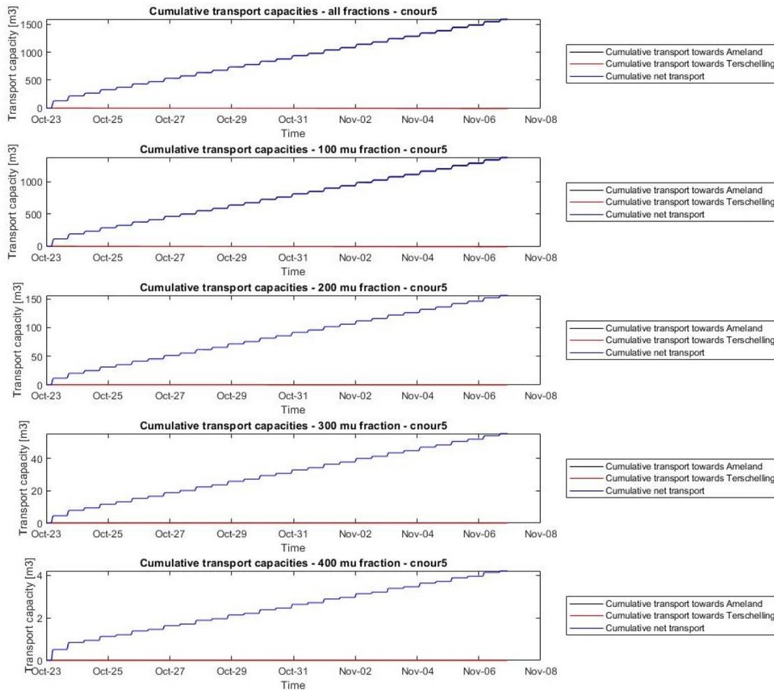
Figure I.10: Tidal transport for all fractions combined and per fraction over a spring neap tide cycle at location cnour5
