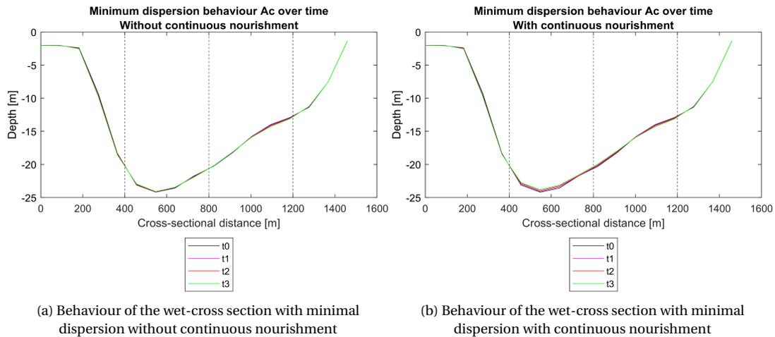
Figure 6.2: Behaviour of the wet cross-section with minimal dispersion. In the left image the behaviour of the wet cross-section is visible in which no nourishment is added over a half year time. In the right image the behaviour of the wet cross-section is visible in which a continuous nourishment is added over a half year time.
