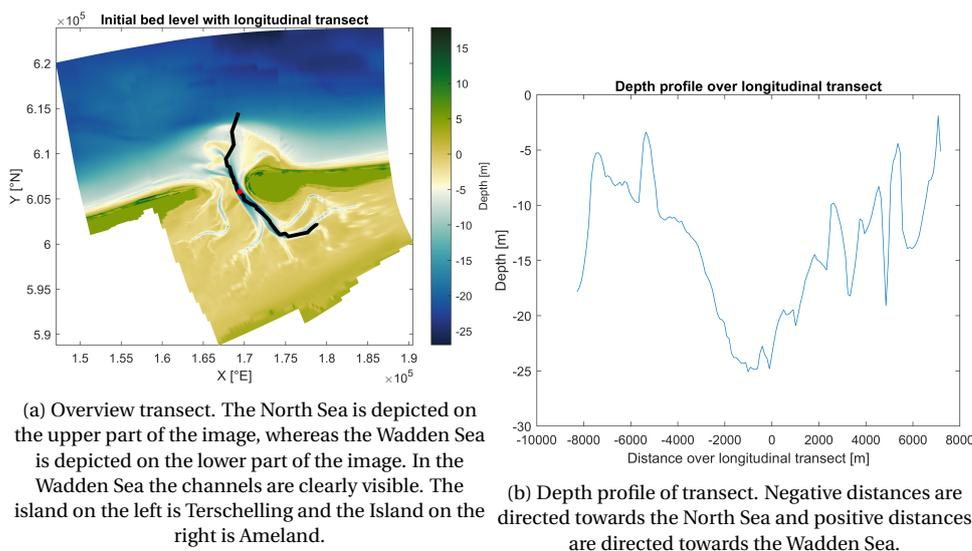
Figure 5.7: Transect and depth profile for the determination of the longitudinal distribution.
