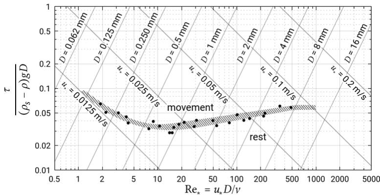
Figure C.1: Shields curve of initiation of motion (Bosboom and Stive, 2021)
