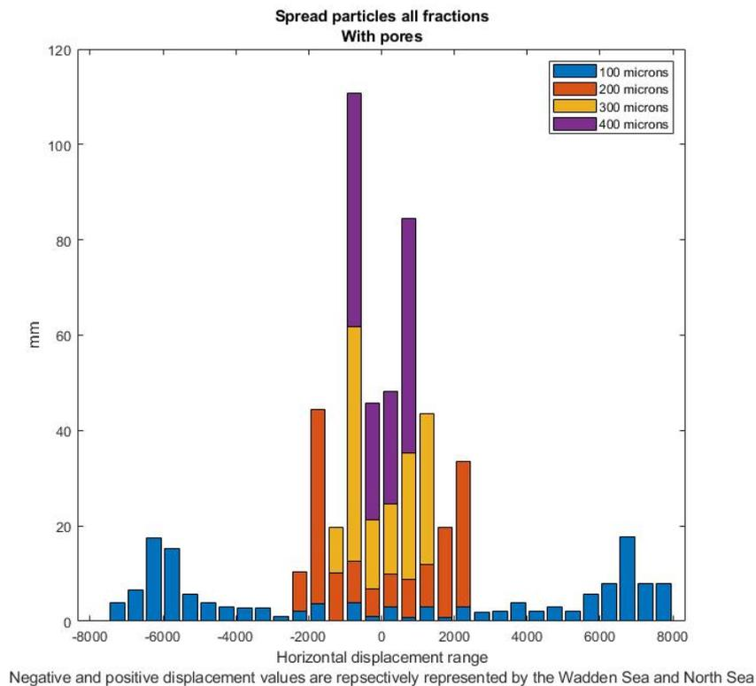
Figure I.12: Increase in bed height determined with the density of sand with pores ( $1600 \frac{kg}{m^3}$ )
