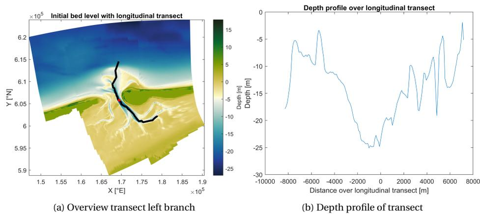
Figure J.5: Transect and depth profile for the determination of the longitudinal distribution
