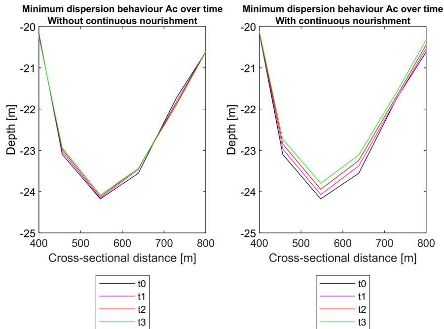
Figure K.2: Behaviour of cross-section over time with a continuous nourishment - Part 2
