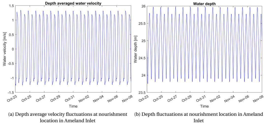
Figure I.2: Water depth and water velocity fluctuations at nourishment location
