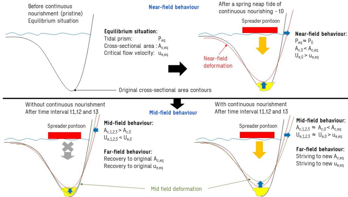
Figure 6.3: Illustrative behaviour of the cross-sectional area due to the continuous nourishment. In the upper row the pristine area is depicted and what happens to the continuous nourishment over a spring neap tide cycle. In the lower row, the response of the cross-sectional area due to the continuous nourishment is depicted for a situation in which the nourishment is stopped and a situation in which the nourishment persists over a half year.
