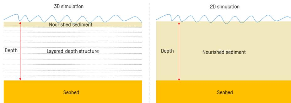
Figure 3.4: Illustration of how the sediment is discharged in the 3D and 2D model.
