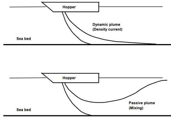
Figure 2.9: Behaviour of Dynamic and Passive plume (van Rijn, 2020)
