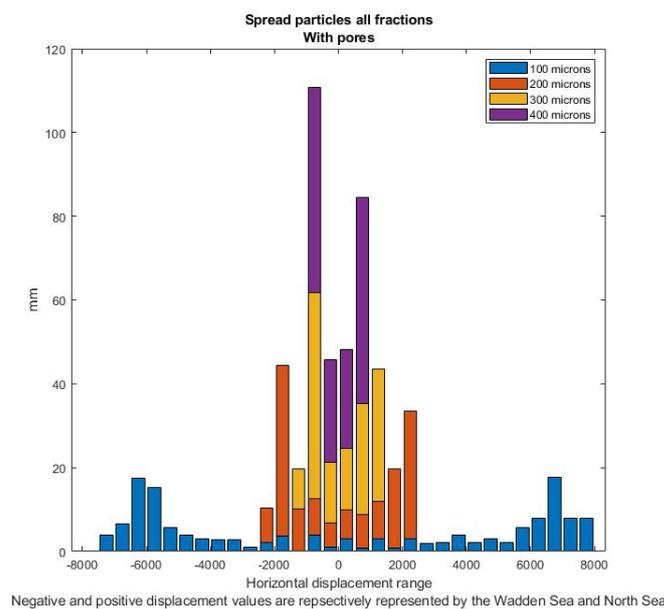
Figure 5.2: Increase in bed height determined with the density of sand with pores ( $1600 \frac{\text{kg}}{\text{m}^3}$ )
