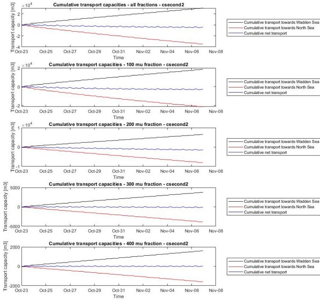
Figure I.9: Tidal transport for all fractions combined and per fraction over a spring neap tide cycle at location csecond2.
