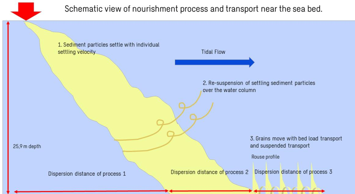
Figure 0.1: Schematic overview of the three dispersion processes. The mixing plume shape originates from (De Wit, 2015)
