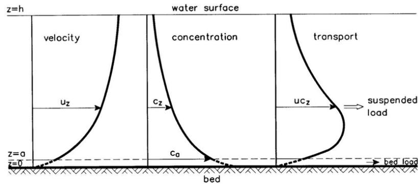
Figure 2.7: Regions of bed load transport and suspended transport (van Rijn, 1993)
