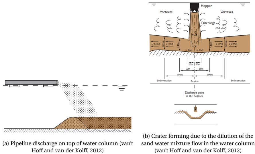
Figure 4.4: Illustration of open pipeline behaviour. This behaviour is undesired as it creates a density driven current to the seabed.
