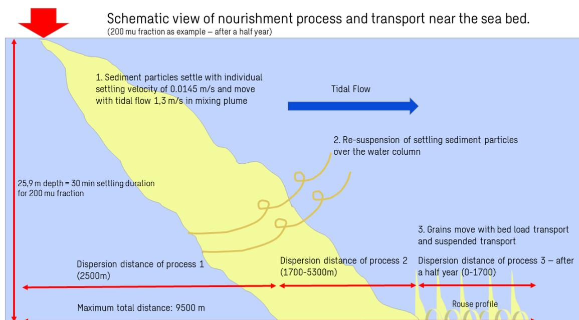
Figure 6.4: Three dispersion processes. This dispersion represents dispersion towards the North Sea. In the mid-field dispersion the focus lies on process 3. This image already has numerical values for the  $200\ \mu\text{m}$  fraction. The results of dispersion process 3 are discussed in this chapter. The dispersion distance of process 1, and 2, are discussed in Chapter 5. The mixing plume shape origins from (De Wit, 2015).
