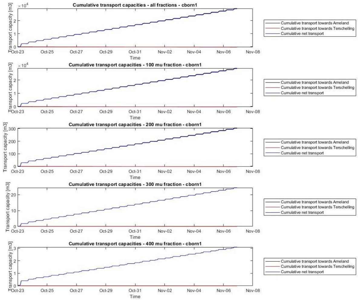
Figure I.7: Tidal transport for all fractions combined and per fraction over a spring neap tide cycle at location cborn1.
