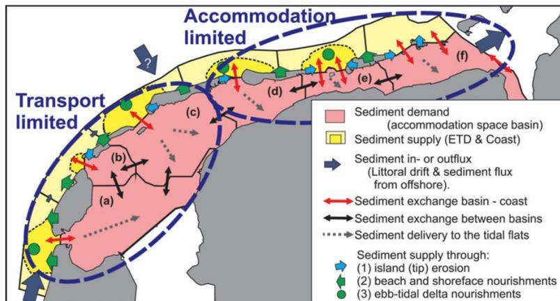
Figure A.5: In the legend; ETD stands for ebb-tidal delta. Schematic overview of the elements, sources, sinks and their linkages that form the sediment-sharing system of the Dutch Wadden Sea. (Wang et al., 2018)
