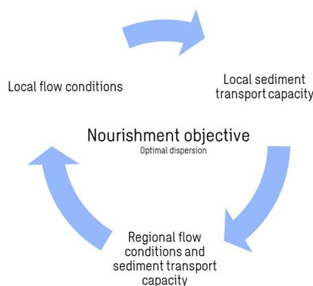
Figure 3.3: Iterative process to determine the exact location of the nourishment.
