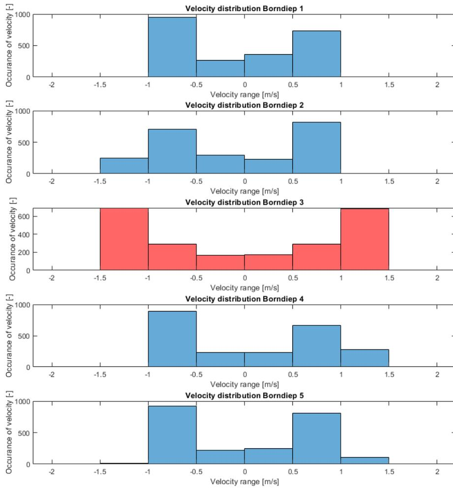
Figure I.3: Velocity distribution over the main channel
