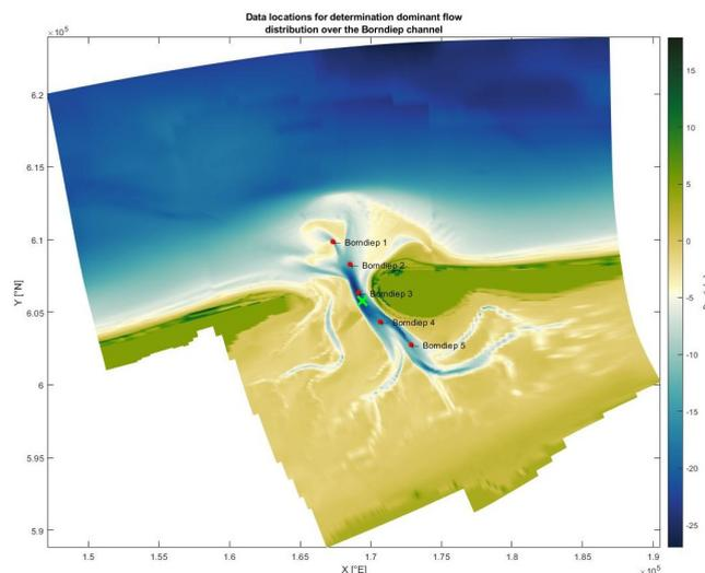
Figure I.1: Locations for further research regarding flow velocities. In red the locations over the Borndiep channel are indicated which are researched in the flow velocity is researched in more detail. In green the chosen nourishment location is depicted.
