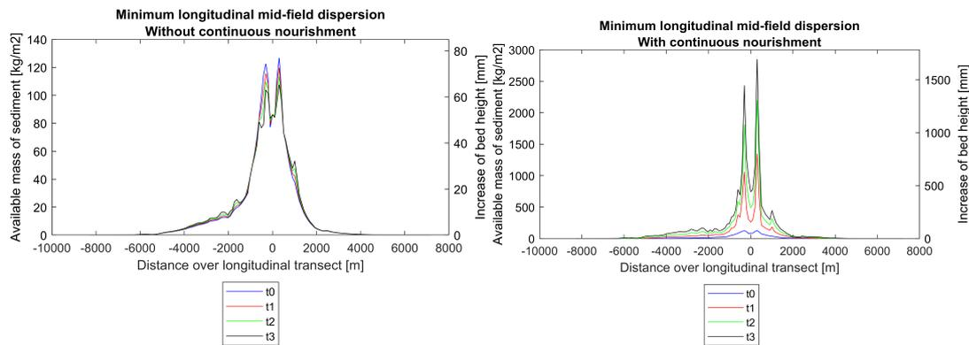
(a) The minimum dispersion over the longitudinal transect per fraction without the addition of a continuous nourishment over a half year. (b) The minimum dispersion over the longitudinal transect per fraction with the addition of a continuous nourishment over a half year.
