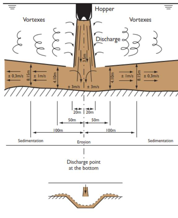
Figure L.2: Crater forming due to the dilution of the sand water mixture flow in the water column (van't Hoff and van der Kolff, 2012)
