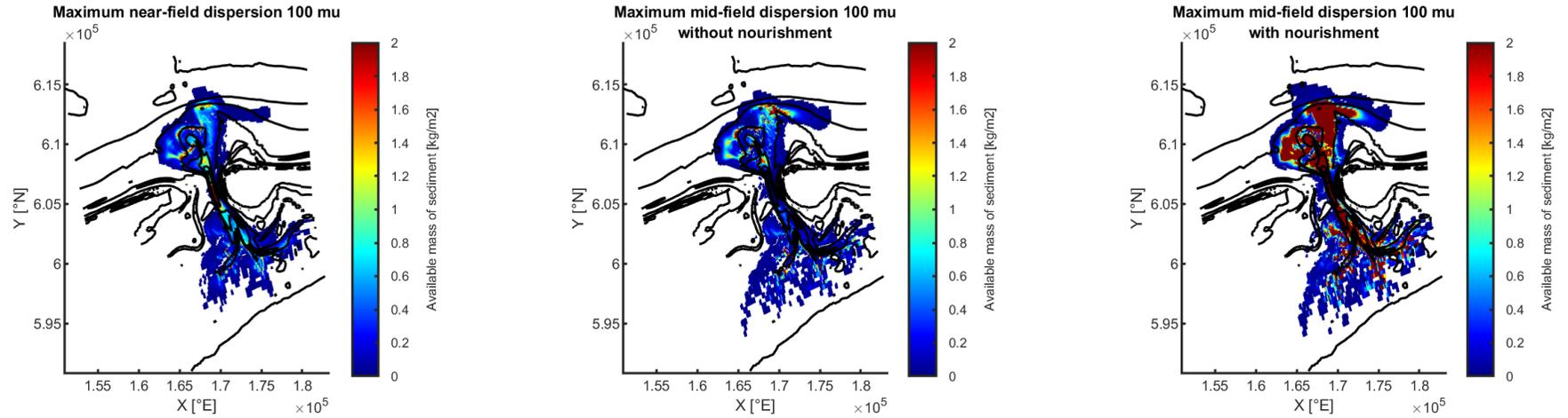
Figure 6.5: Combined figures of maximum dispersion. 3D spring neap tide cycle (left), 2D half year dispersion without continuous nourishment (center) and 2D half year dispersion with continuous nourishment (right) - 100 $\mu$ m
