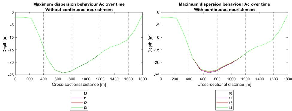
(a) Behaviour of the wet-cross section with maximal dispersion without continuous nourishment
