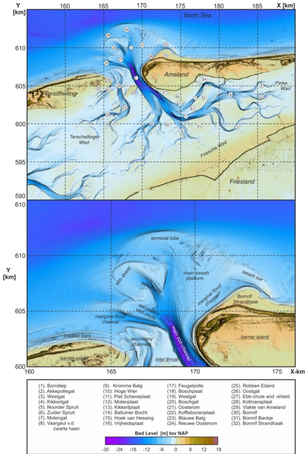
Figure A.2: Upper image: Amelander zeegat with a grid and numerical values to indicate locations. Lower image Components of a tidal Inlet system. The image is obtained from (Elias, 2017)
