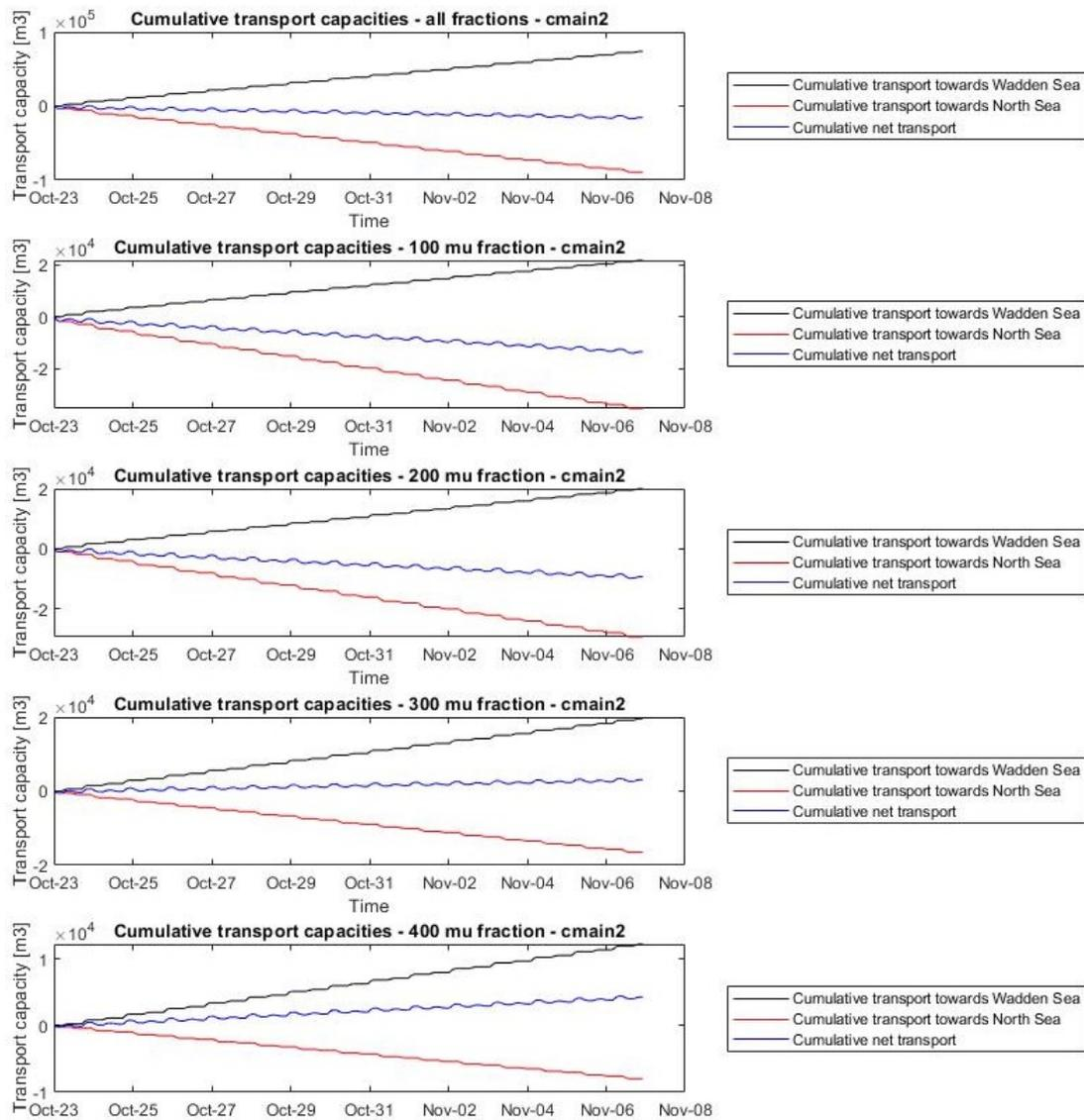
Figure I.6: Tidal transport for all fractions combined and per fraction over a spring neap tide cycle at location cmain2.
