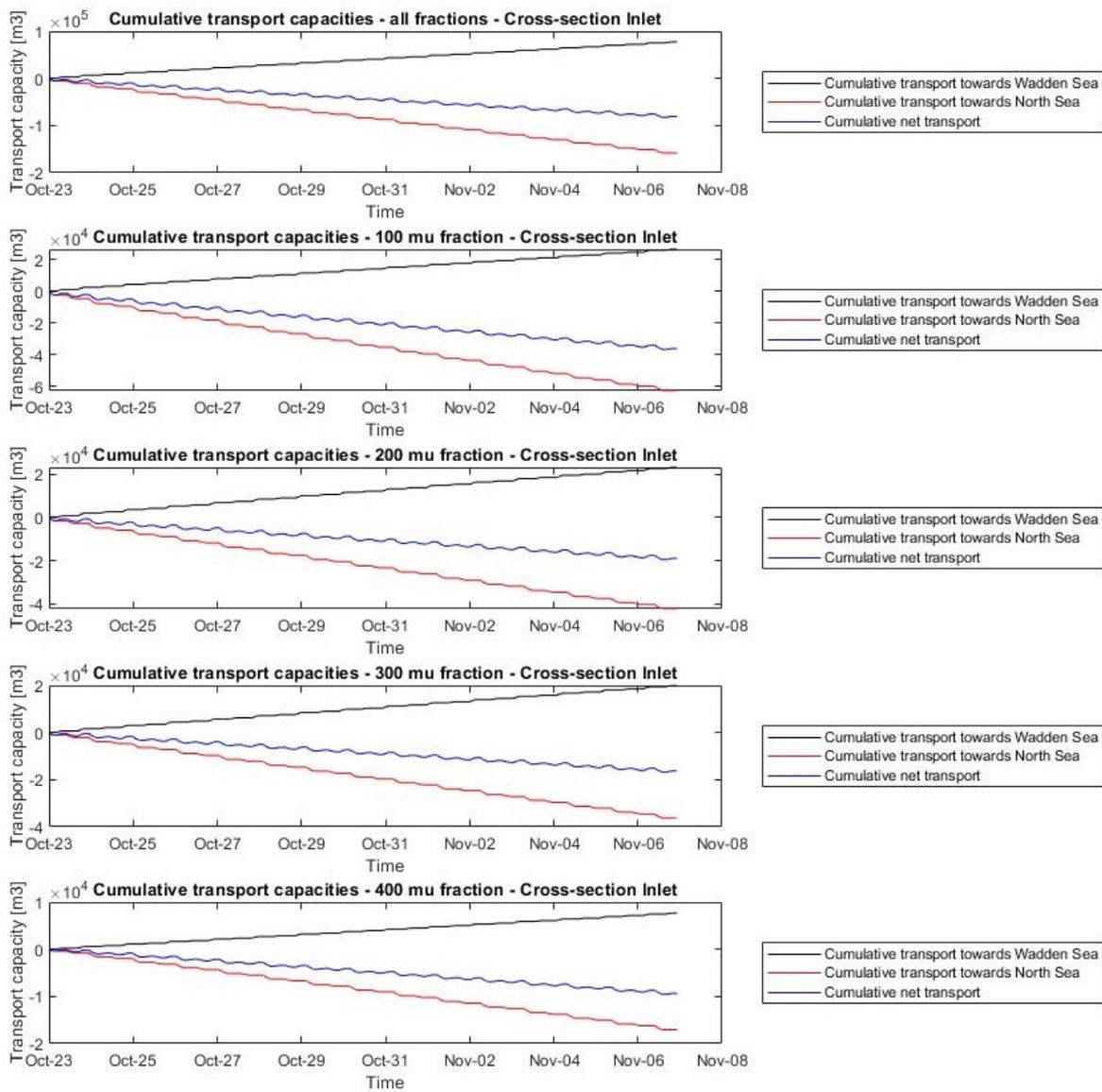
Figure I.5: Tidal transport for all fractions combined and per fraction over a spring neap tide cycle over the Inlet
