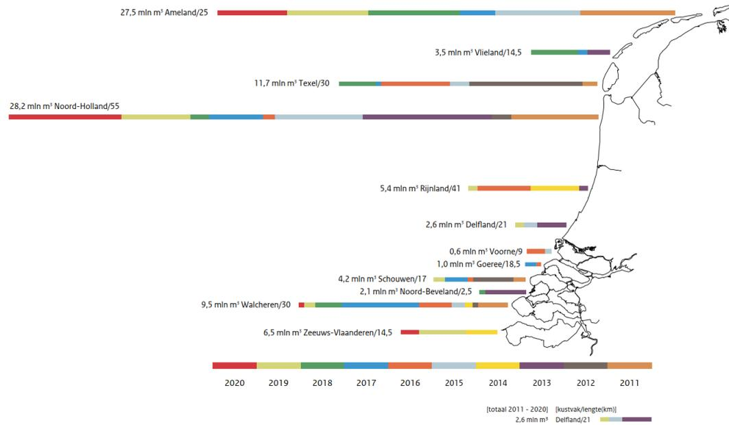
Figure 1.1: Coastline nourishment overview. Total amount of executed sand nourishments in  $Mm^3$  in the period of 2011-2020. The image is obtained from (Rijkswaterstaat et al., 2020)
