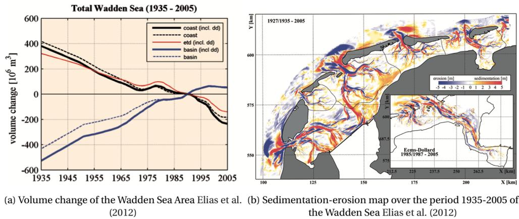
Figure A.4: Volume change and erosion and sedimentation maps
