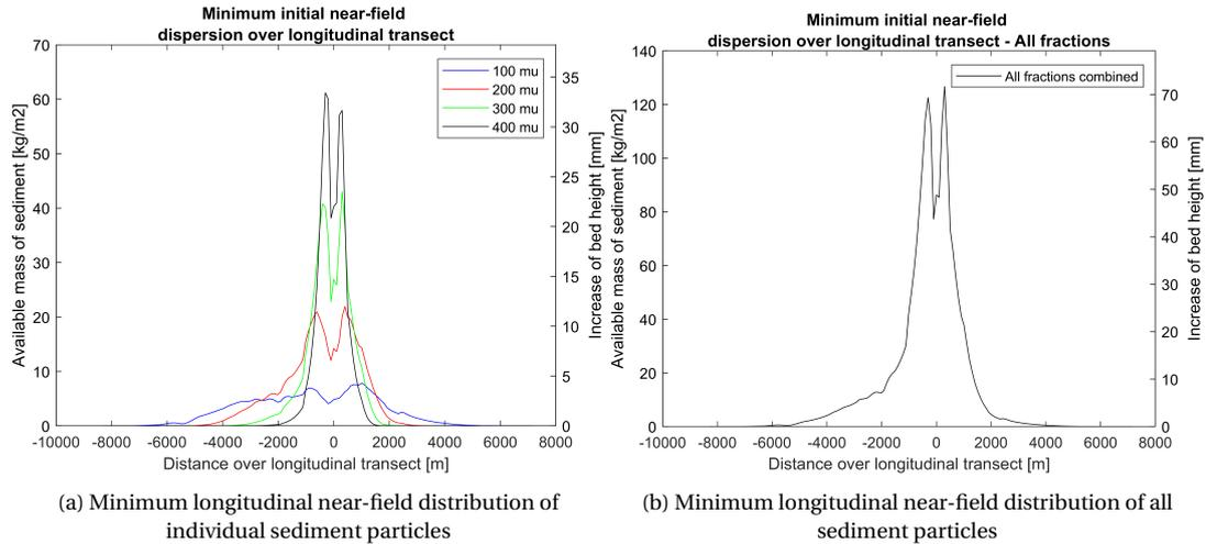
Figure 5.8: Longitudinal transect of minimum near-field distribution. The longitudinal transect is taken through the tidal channel as depicted in Fig. 5.7a.
