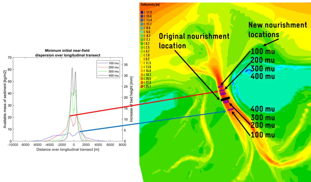
Figure H.2: Overview of how the longitudinal distribution is used to determine the new nourishment locations.
