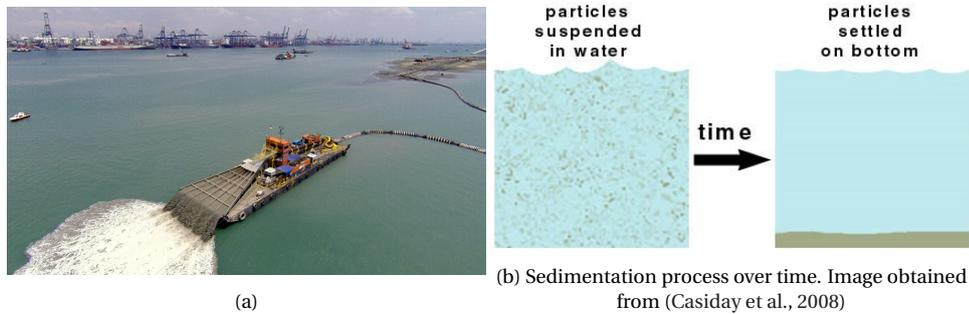
Figure 4.5: In the left image an example of the spreader pontoon is illustrated. In the right image the process over time which is desired to obtain by placing the sediment as a mixing plume is illustrated.
