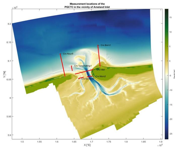
Figure I.4: Locations in the vicinity of Ameland Inlet where the tidal sediment transport is determined.
