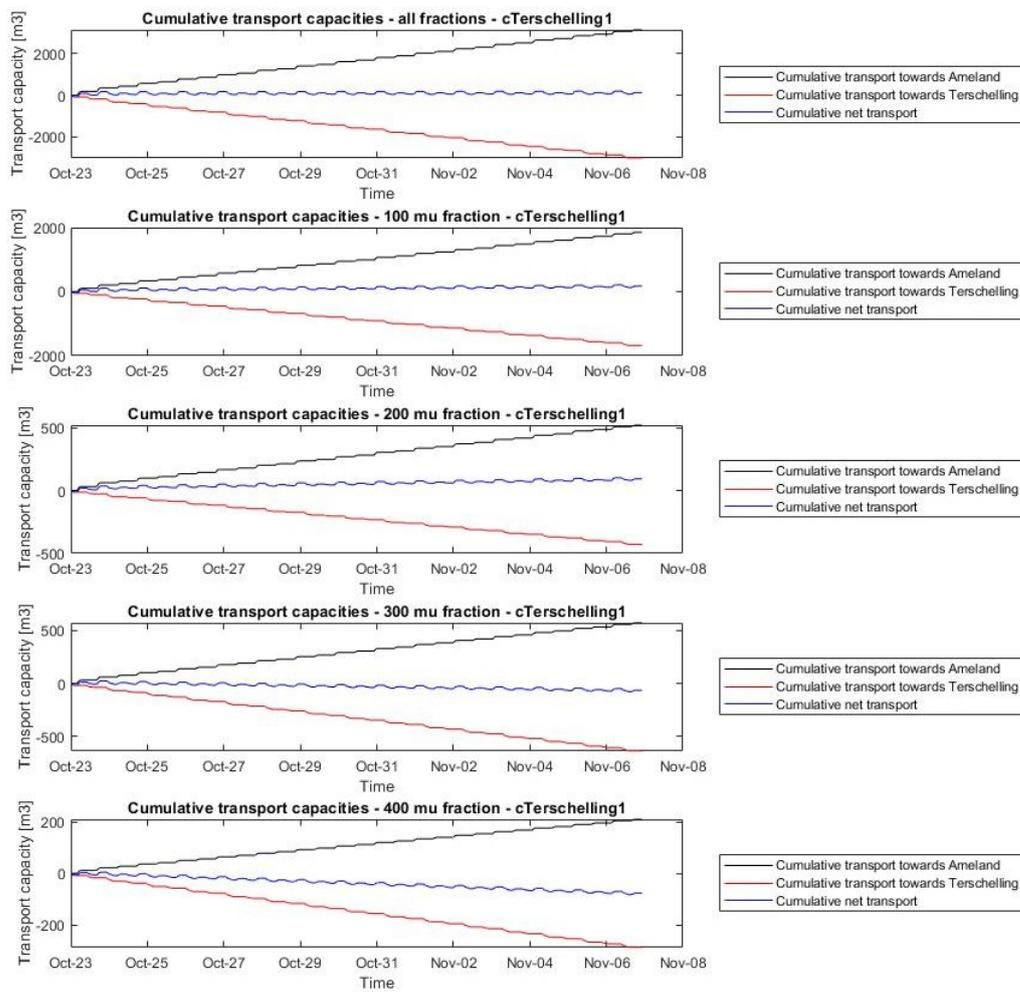
Figure I.8: Tidal transport for all fractions combined and per fraction over a spring neap tide cycle at location cterschelling1.
