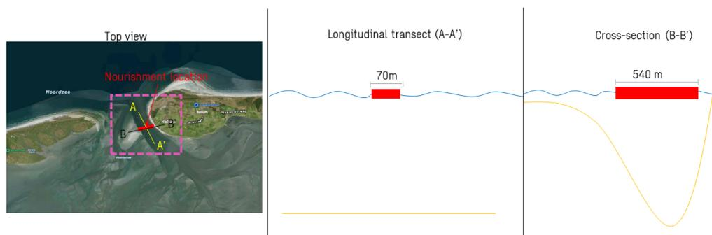
Figure 4.3: Nourishment strategy. Left figure is a top view of where the nourishment is executed. In red the nourishment area is depicted. In the center figure, the length over which the nourishment is spread out is depicted. In the right figure, the width over which the nourishment is spread is depicted.
