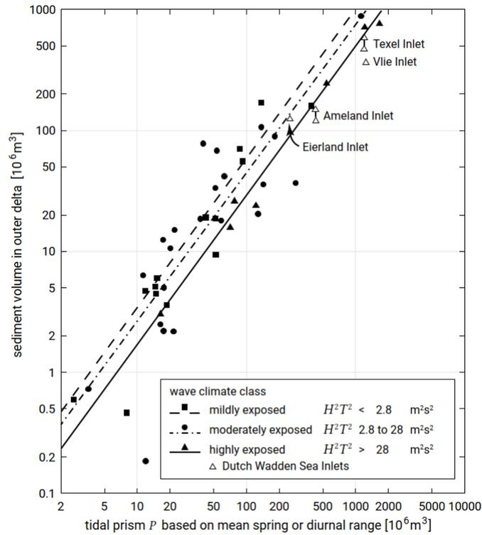
Figure B.1: Empirical relationship between volume of sand in the outer delta and the tidal prism (Bosboom and Stive, 2021)
