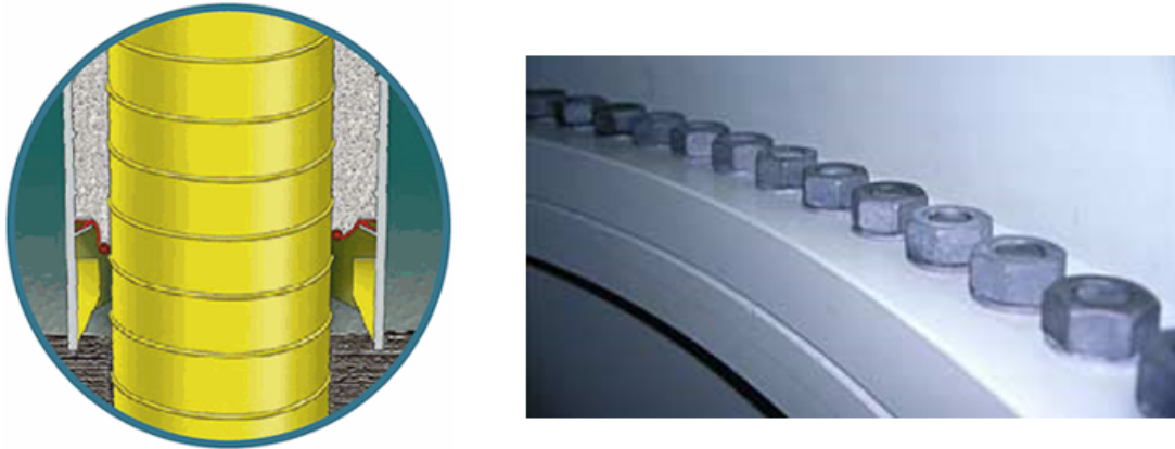
Figure 1.2: Left: grouted connection [8], Right: bolted connection [34].
