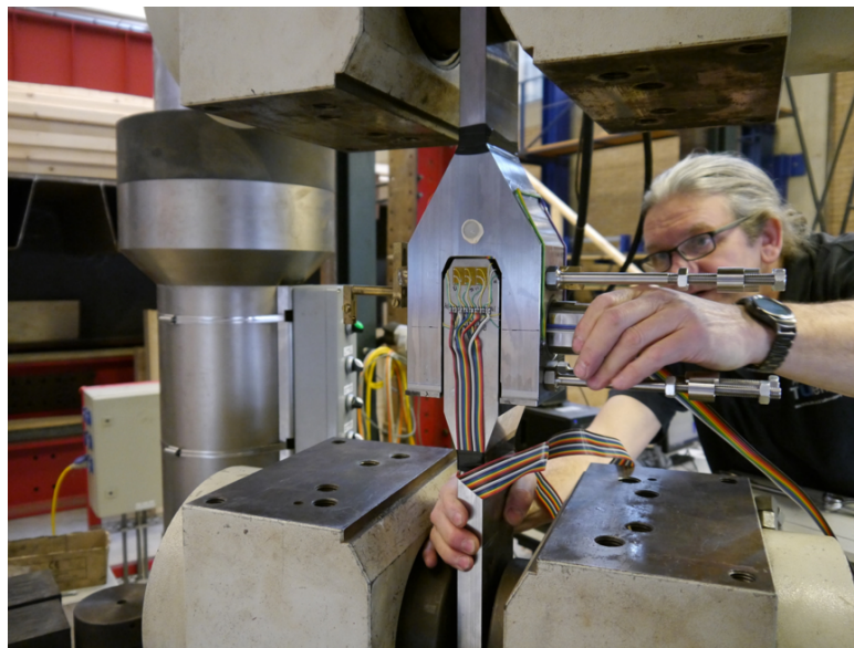
Figure 6.8: Tested segment of wedge connection under fatigue loading.
