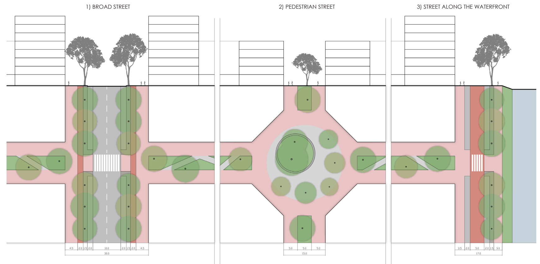
Three types of street profiles, scale 1:1000.
